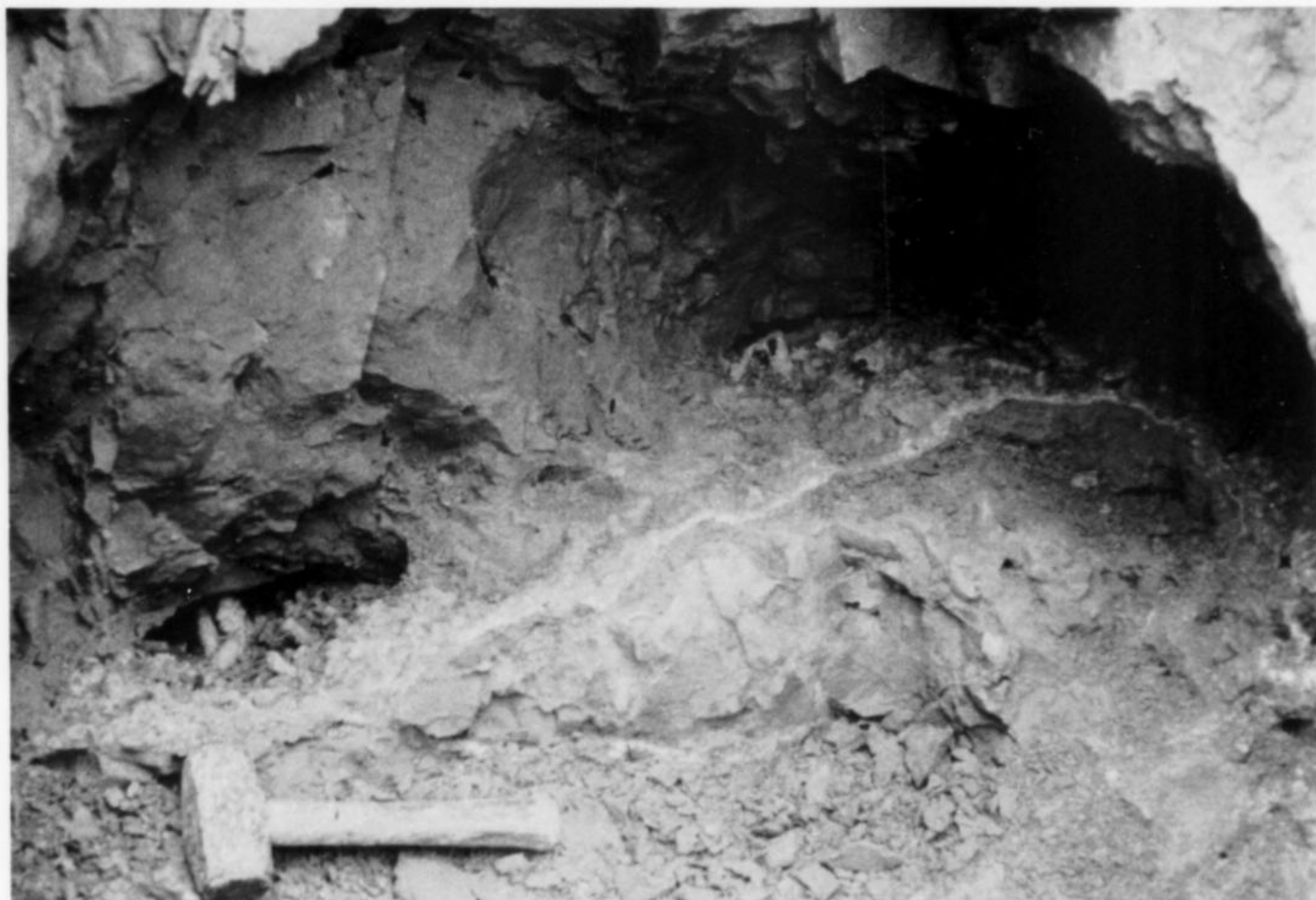
Figure 8. Two pockets in the calcite seam; a pinched out zone separates them.
