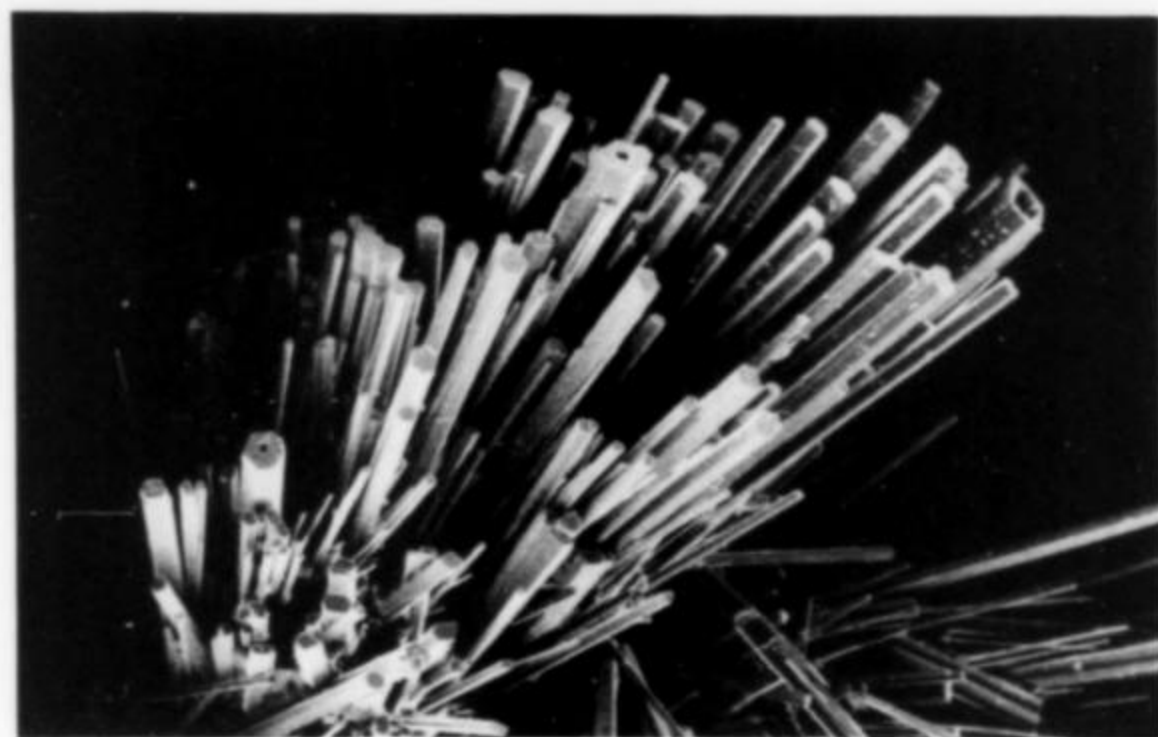
Figure 32. SEM photomicrograph of a tiptopite spray showing the cavernous nature on a few of the crystals.
