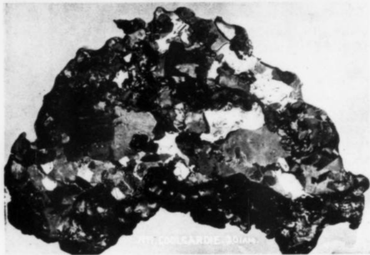
Figure 31. Etched and polished section of a 4-cm gold nugget from Coolgardie, Western Australia, showing crystalline interior (from Liversidge, 1894, plate 4).
