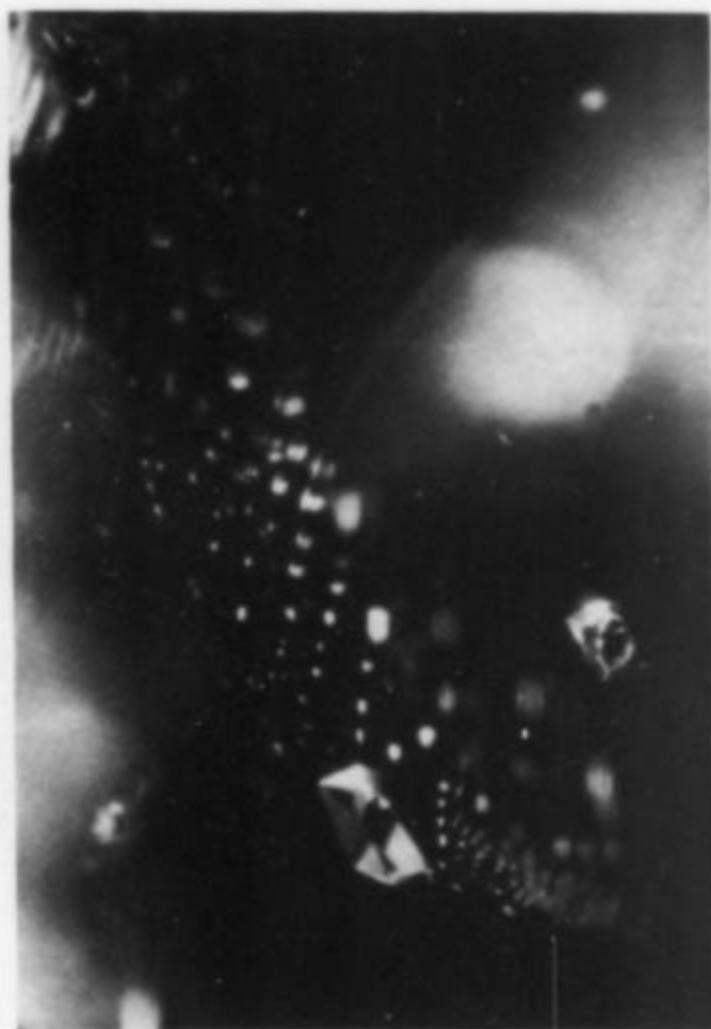
Figure 16. A veil of liquid inclusions and negative crystals within a colorless quartz crystal from Fonda, Montgomery County, New York. Field of view, 2.5 mm.
