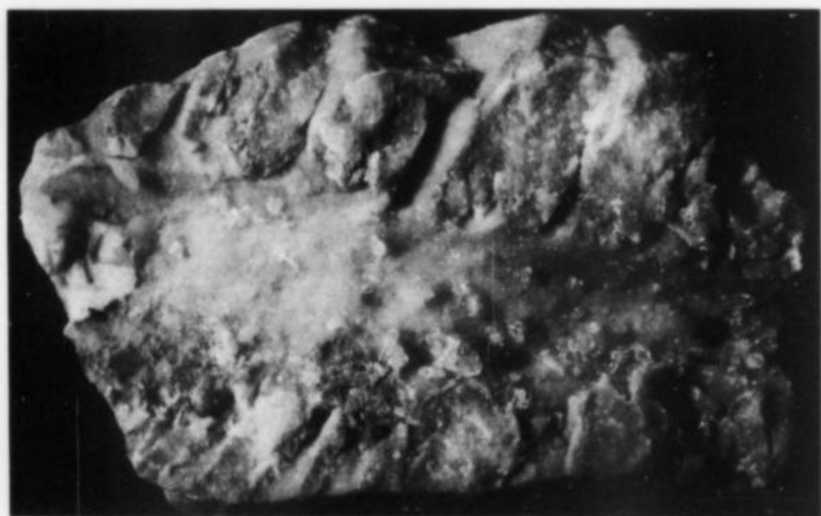
Figure 88. Elongated cavity with typical lateral tension fractures 14 cm. University of Pisa collection, Gini photo.
