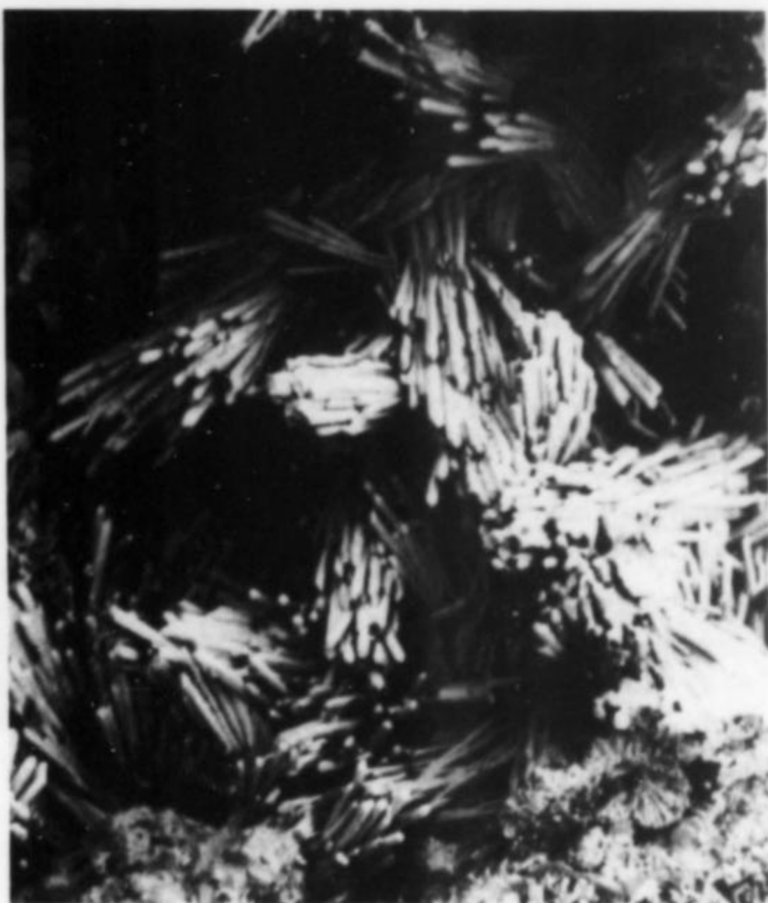
Figure 5. Bundles of acicular, carmine-red carminite crystals filling cavities in gossan, average size 0.01 x 1.5 mm. Dunning SEM photo and specimen.
