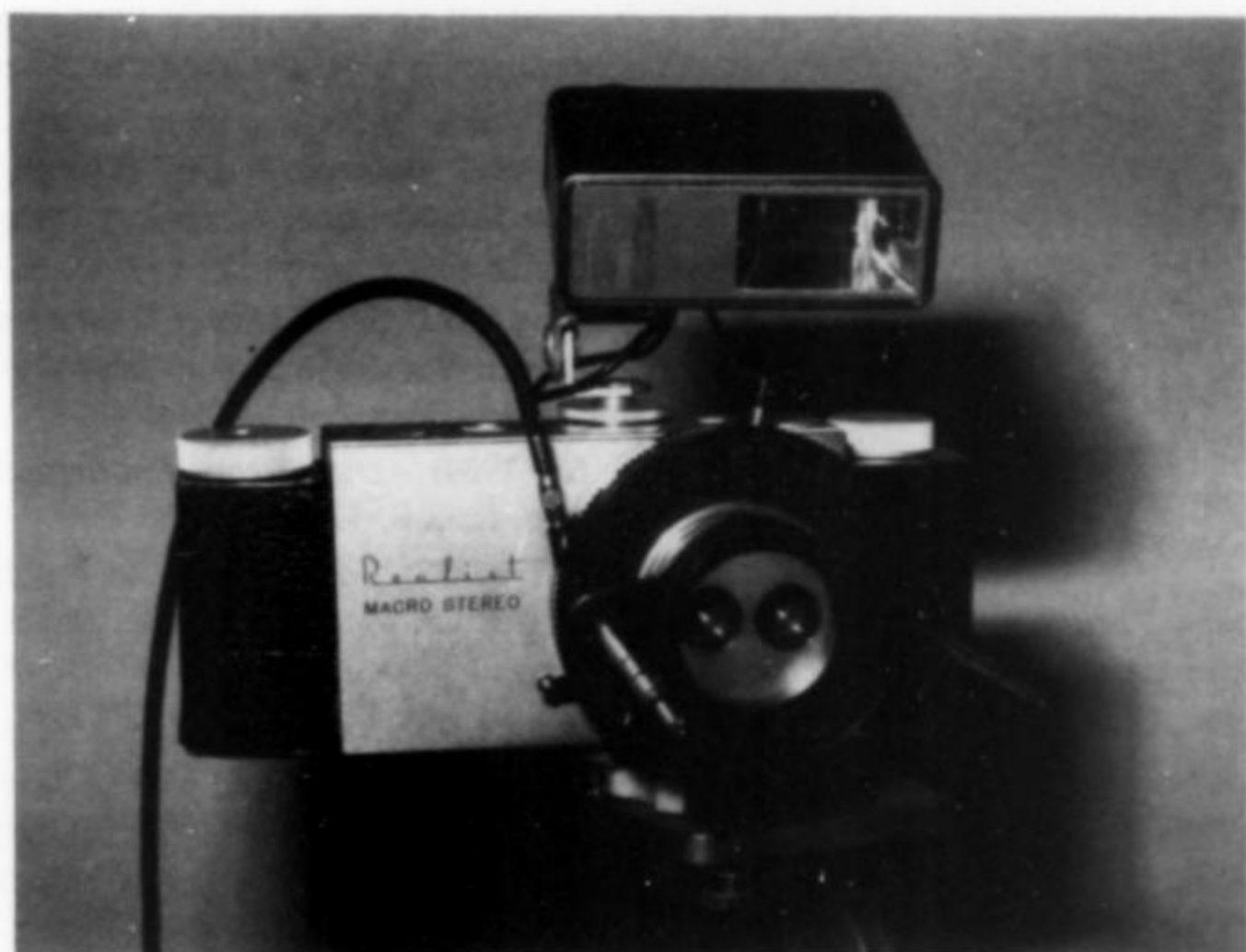
Figure 9. The Realistic macro stereo camera for close-up work. (Courtesy of David Huddle.) The two photos are taken simultaneously, so that no rotation of the specimen between shots is necessary.
