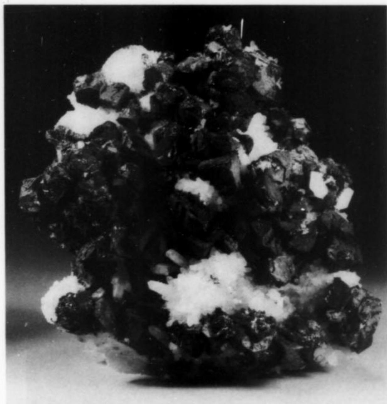
Figure 8. Galena and sphalerite; Mountain Monarch mine. Small cubes modified by octahedral faces. Individual crystals to 7 mm; 6 x 7 cm overall.
