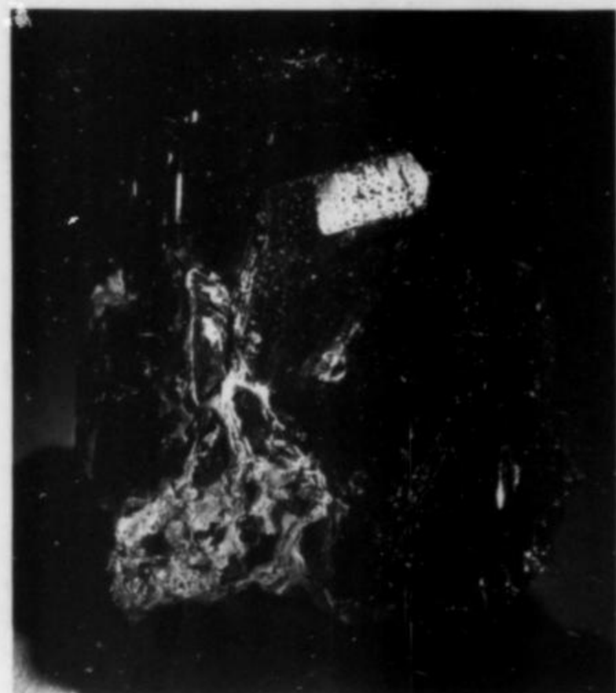
Figure 6. Barite with chalcopyrite inclusions from the Black Rock open cut, Mount Isa mine. The specimen is 10 cm tall. Museum of Victoria collection; photo by Frank Coffa.
