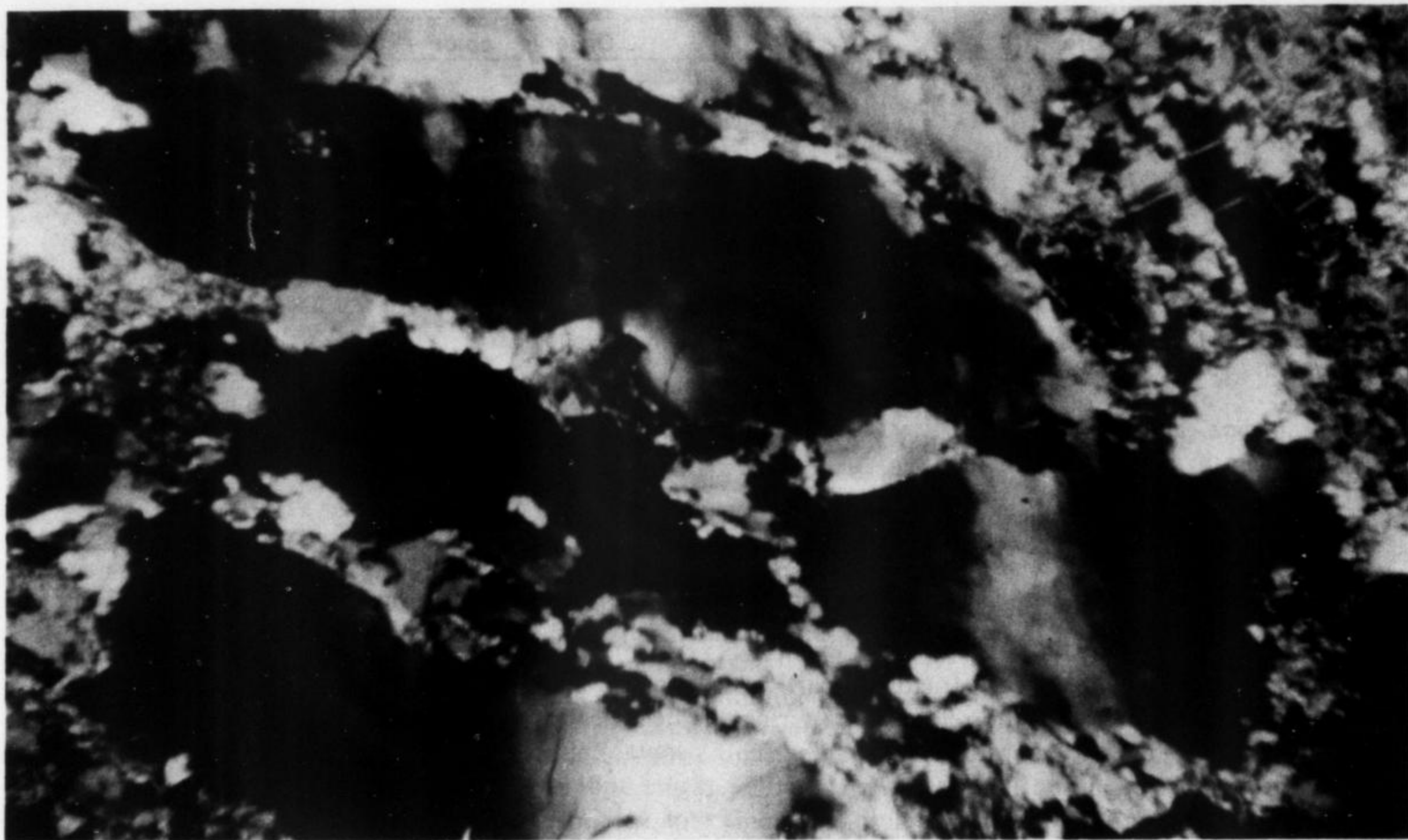
Fig. 2. Photomicrograph of microfractured and strained quartz: crossed nicols; longer, horizontal dimension of plate is approximately 18 mm.
