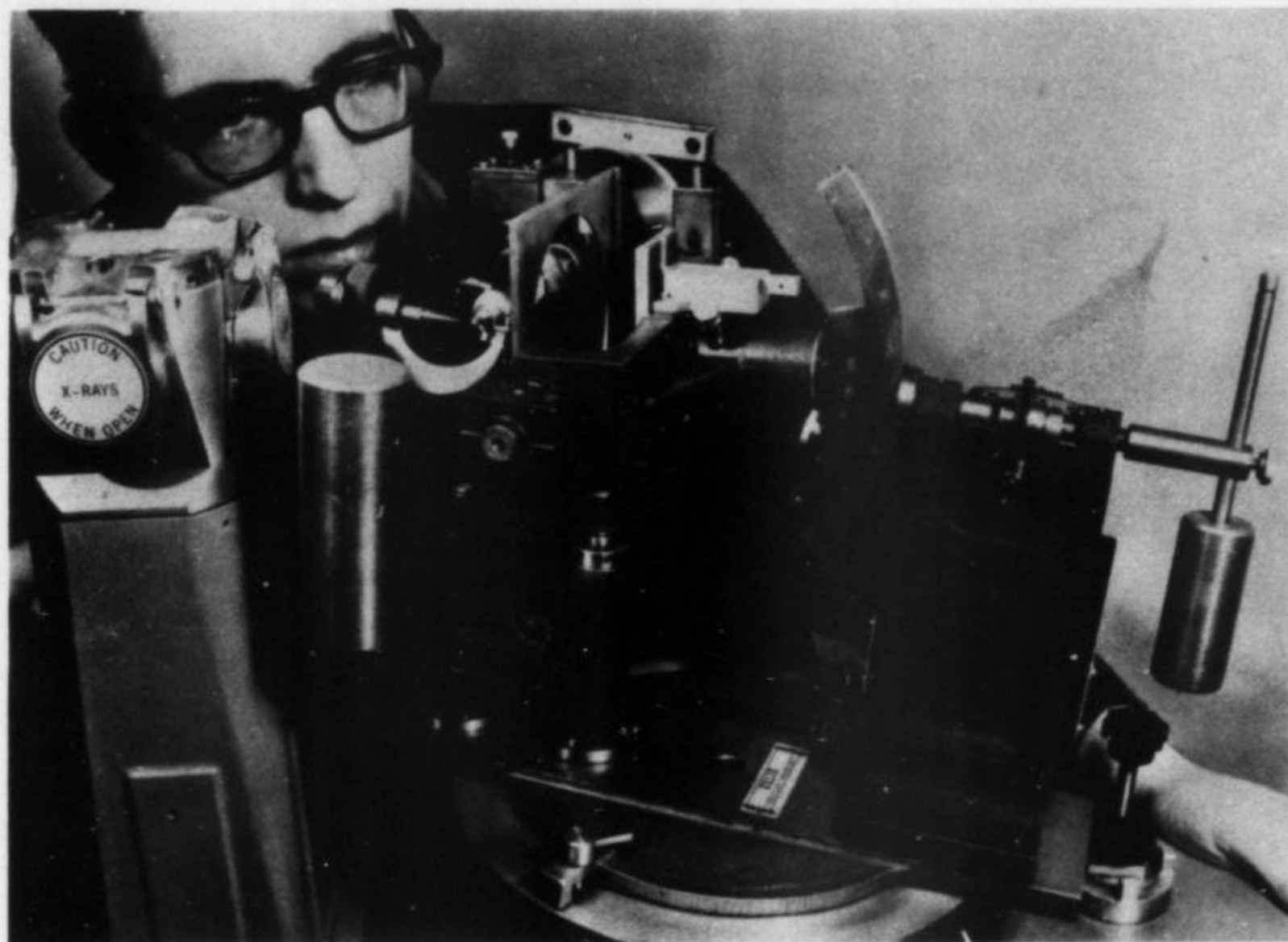
Fig. 12. The author is shown aligning a crystal on a Buerger Precession camera. The rather complex gear mechanisms on this camera eliminate the distortions of the Weissenberg technique, and give direct, angle-true views of crystal symmetry.
