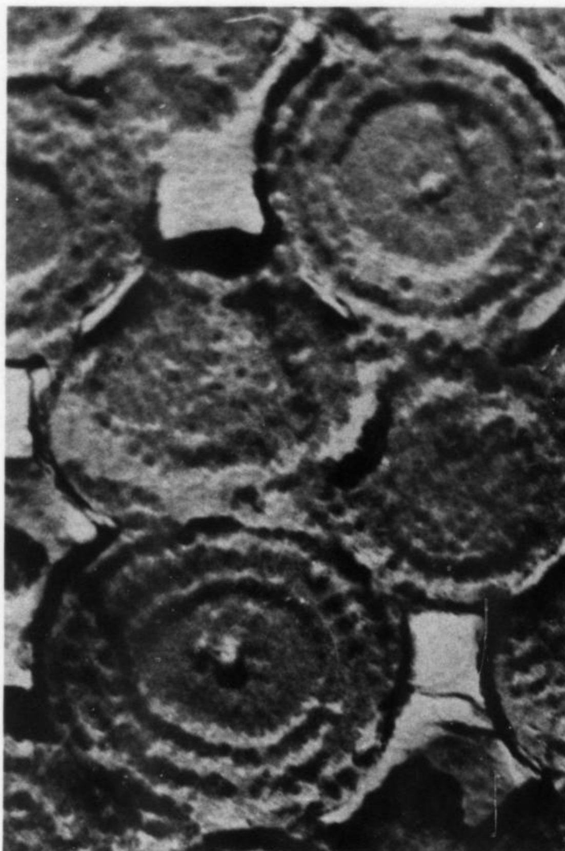
Fig. 6 Lightly etched surface of opal showing the internal structure of shells within the particles. In the two biggest sections at the top and bottom the outer three shells only can be seen. The inner ones have not been etched. Shaded replica, x 70,000.
