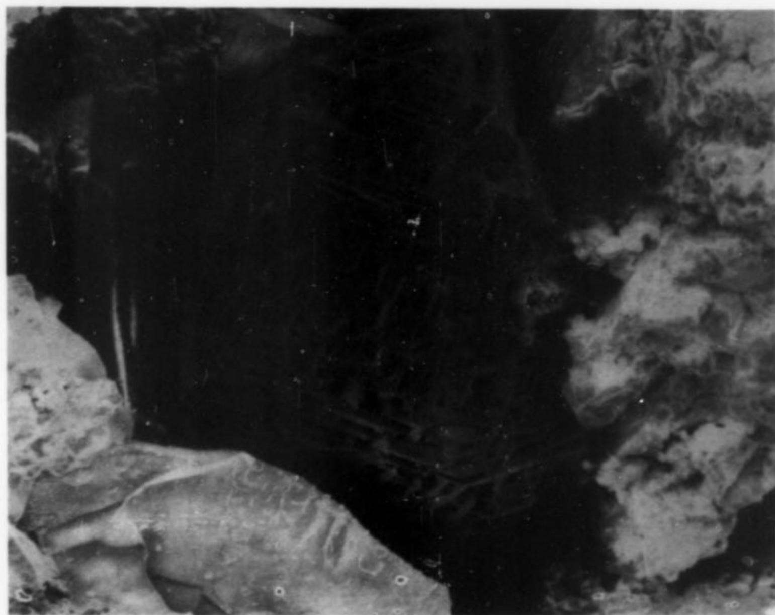
Figure 2. SEM photograph of multiple ridges of ilmenite epitaxial on bixbyite. Viewed down a [100] axis, crude cube and octahedron faces of the bixbyite are discernible. Size of crystal, 0.6 mm.
