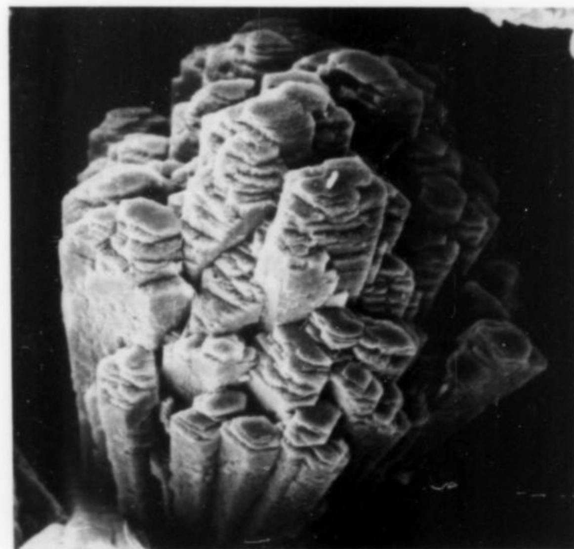
Figure 12. SEM photomicrograph of end of aggregate of dufrenite shown in Figure 11. Note the buildup of successive plates. Aggregate is 0.28 mm across.
