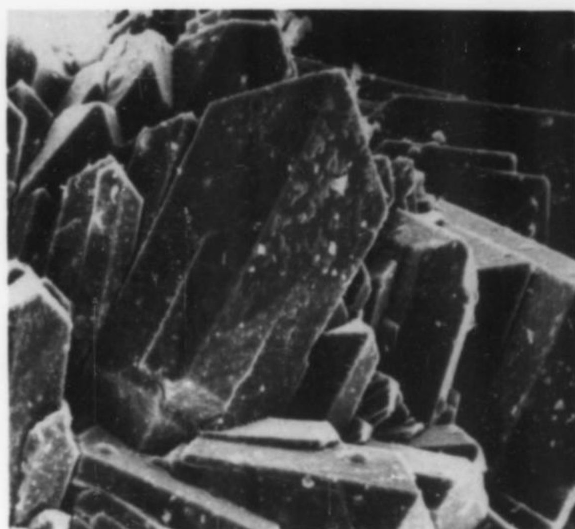
Figure 21. SEM photomicrograph of transparent yellow strengite from Rock Run Station, Alabama. The largest crystal has a length of 0.125 mm.
