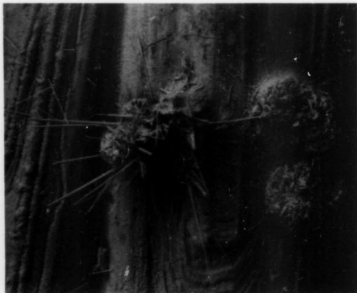
Figure 11. SEM photo of a stibiconite pseudo-morph after stibnite with small needles of valentinite, 0.04 mm in diameter. G. Dunning specimen and photo.
