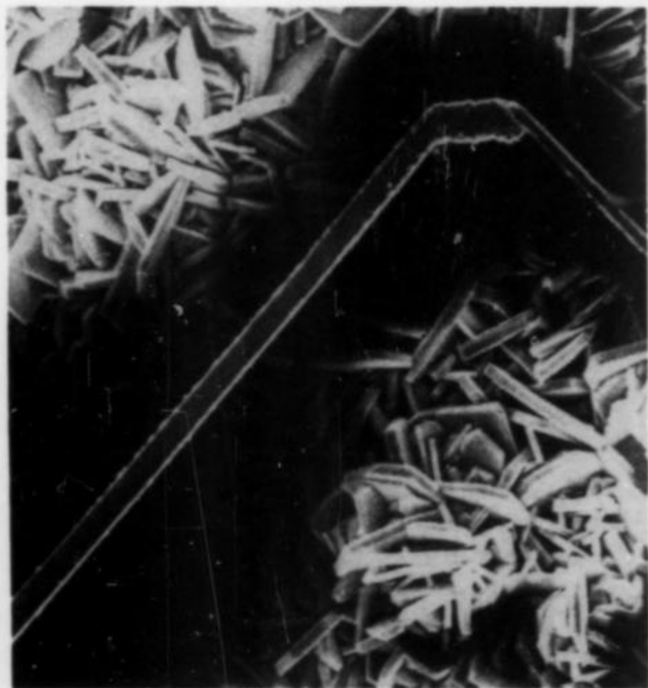
Figure 6. SEM photo showing 45° bends in pyrite from Clackamas River, Oregon. Field of view, 0.6 mm; Violet Frazier specimen.
