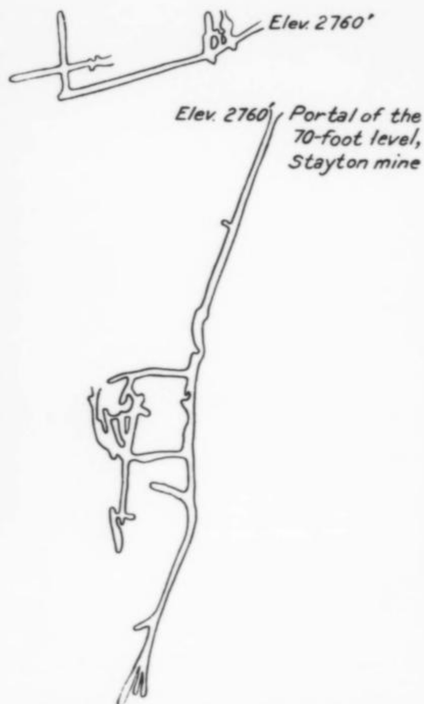
Figure 6. Underground map of the Stayton mine showing the location of extensive stoping for stibnite and cinnabar (after Bailey and Myers, 1941).
