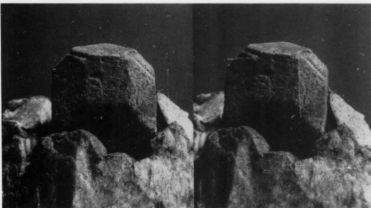
Figure 24. Blocky crystal of antiperthite 2.5 cm wide. Orientation is indicated by the topmost face, the basal pinacoid {001}, all others being back-of-crystal faces. National Mineral Collection of Canada. Stereo-pair photo by the author.
