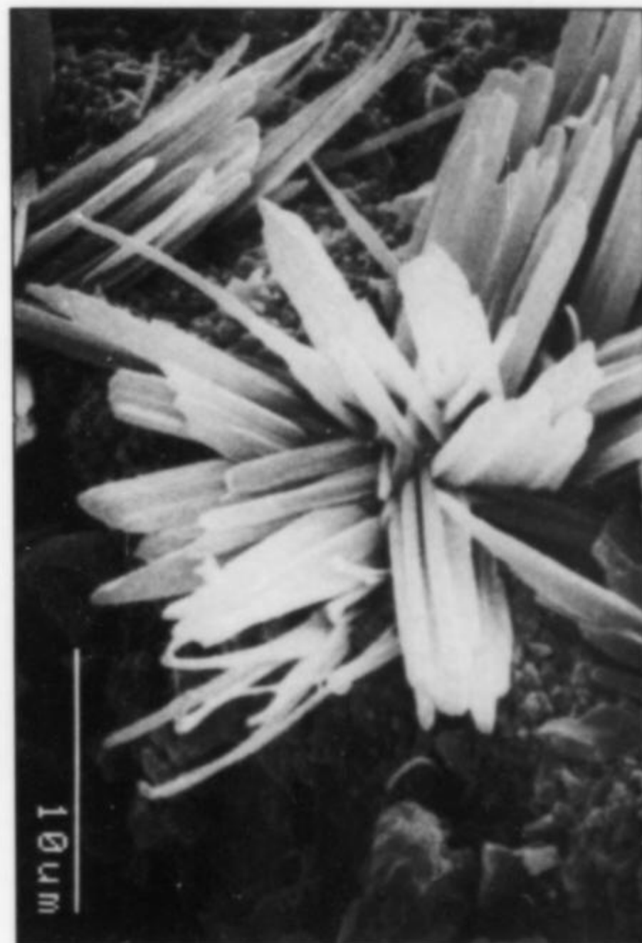
Figure 22. Britholite-(Ce), a radiating group of crystals. The needles are 10 to 15 microns in length. National Museum of Natural Sciences (Canada) specimen #53747. SEM photo by I. Wainwright.
