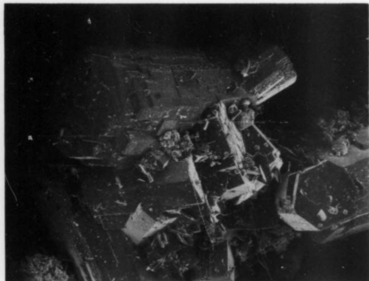
Figure 1. SEM photograph of zanazziite crystals, showing the common pseudo-hexagonal morphology. The largest crystal is about 0.4 mm in length. NMNH #R17847.
