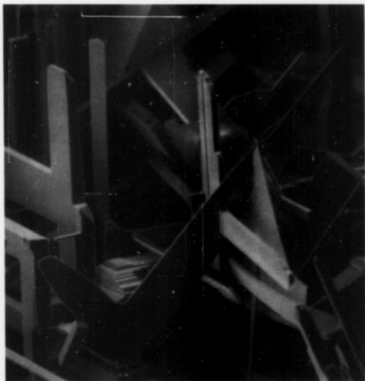
Figure 39. Filiform pyrite showing elongated crystals in a three-dimensional orthogonal reticulation, with "goalie sticks." Scale bar 50 microns long. CMN #MOC3323. SEM by G. W. Robinson.
