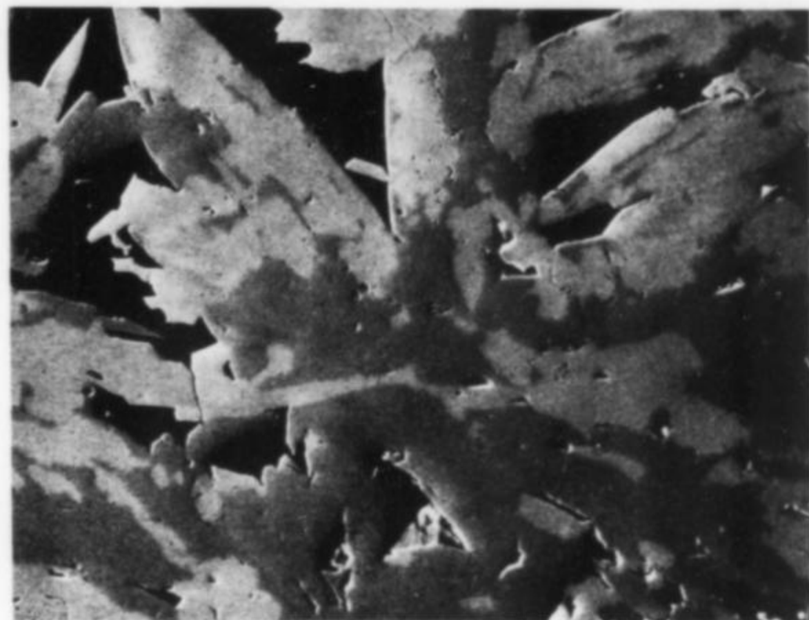
Figure 15. Backscattered electron image of a polished section of iron ore from the Middleback Range in South Australia showing intergrown hematite (dark) and magnetite (light). The difference in average atomic number between these two minerals is around 0.5 absolute. Field of view is 0.7 mm across. Author's specimen and micrograph.
