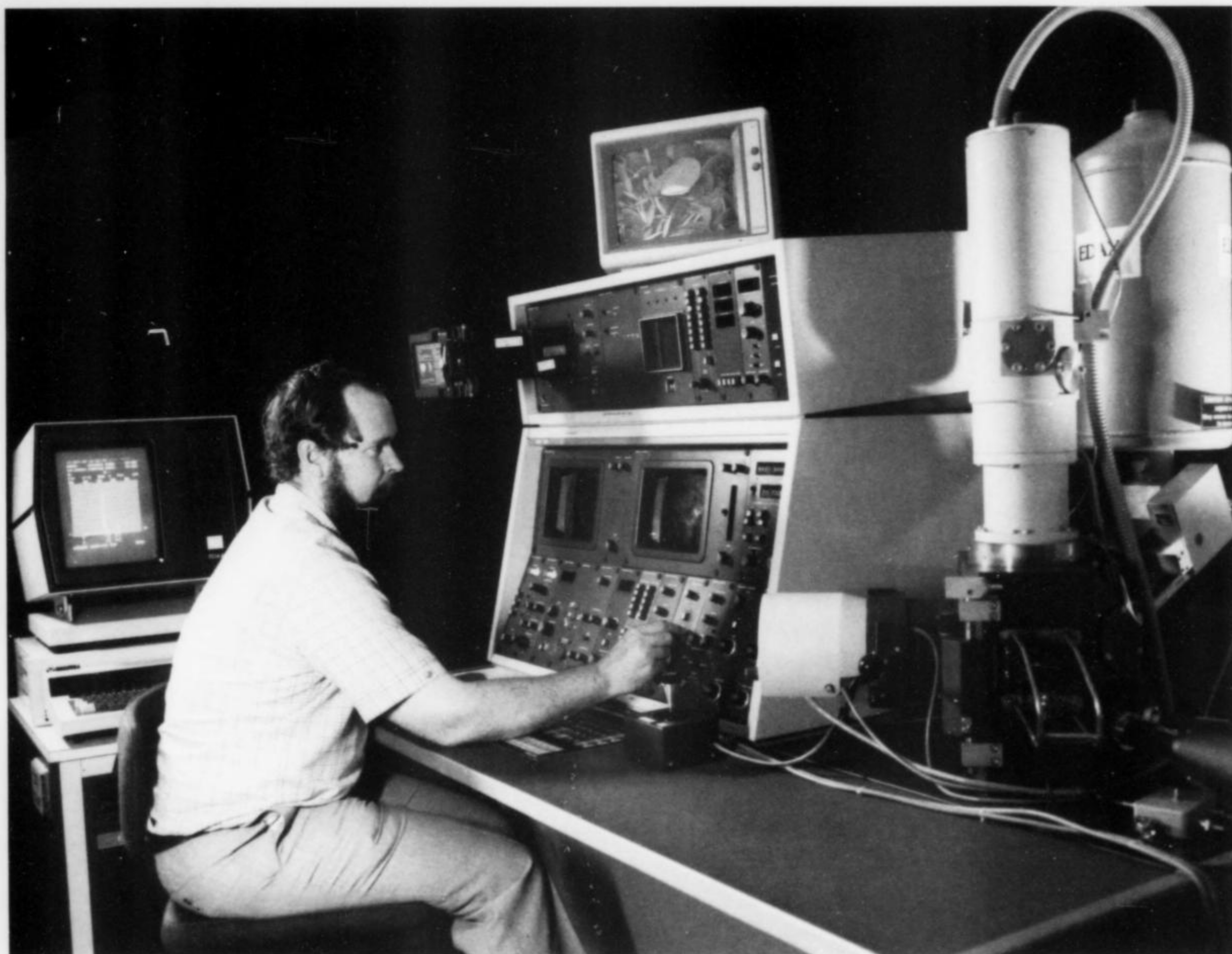
Figure 1. An example of a modern scanning electron microscope. The Philips SEM505 installed at the Newcastle Laboratories of Broken Hill Proprietary Co. Ltd. Research Division. Photo by Murray McKean of the Newcastle Laboratories Photography Group.
