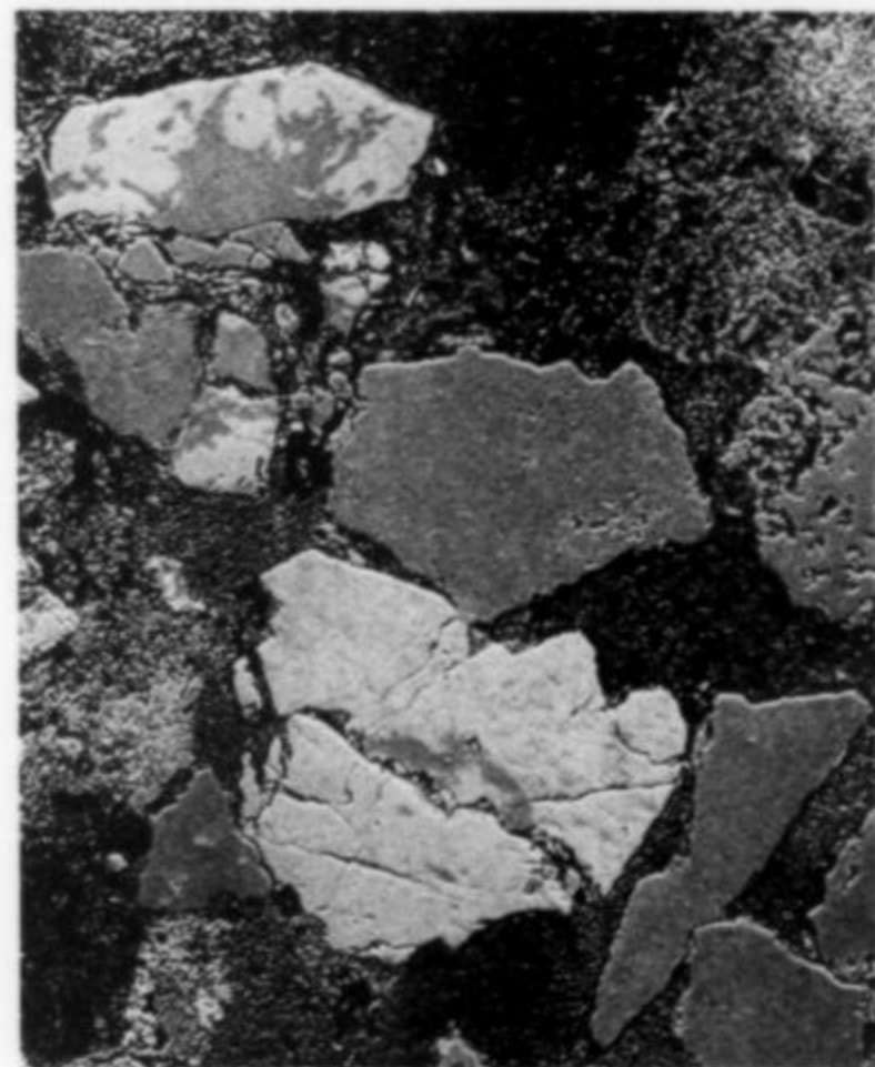
Figure 17. Greywacke from the Hunter Valley, New South Wales. Backscattered electron image of a polished section showing angular grains of quartz (gray) and albite/K-feldspar (mottled) in a fine kaolinite matrix. Field of view is 1 mm across. Author's specimen and micrograph.
