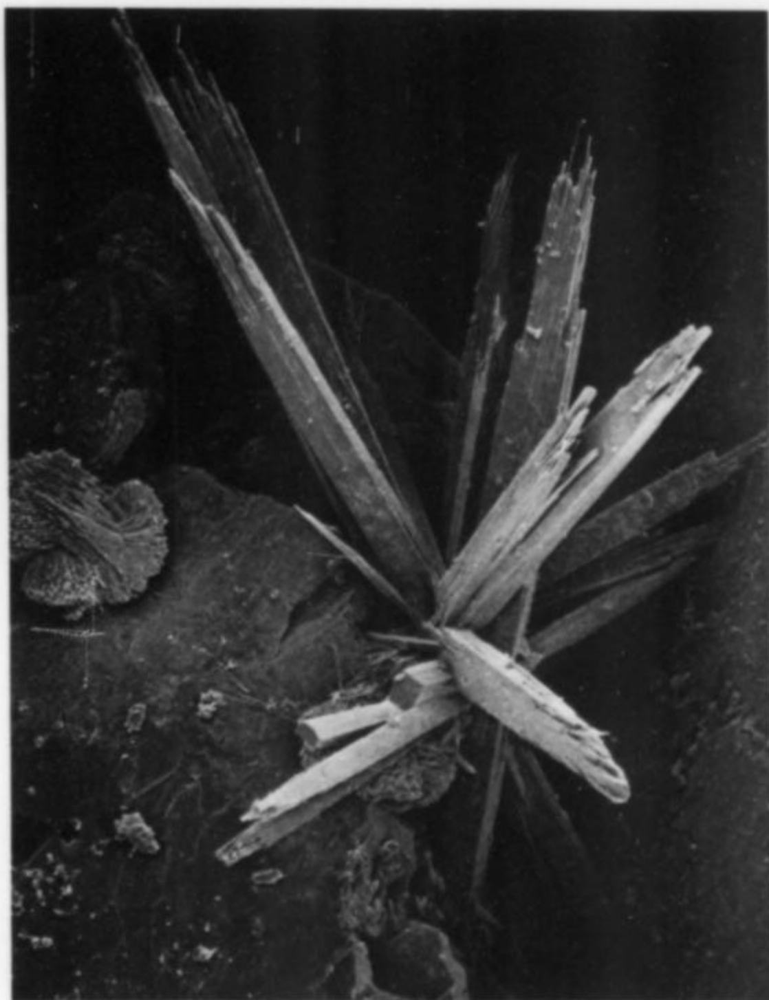
Figure 7. Crystals of ulrichite on quartz from the Lake Boga granite quarry, Victoria. Secondary electron image. Field of view is 0.5 mm across. Author's specimen and micrograph.
