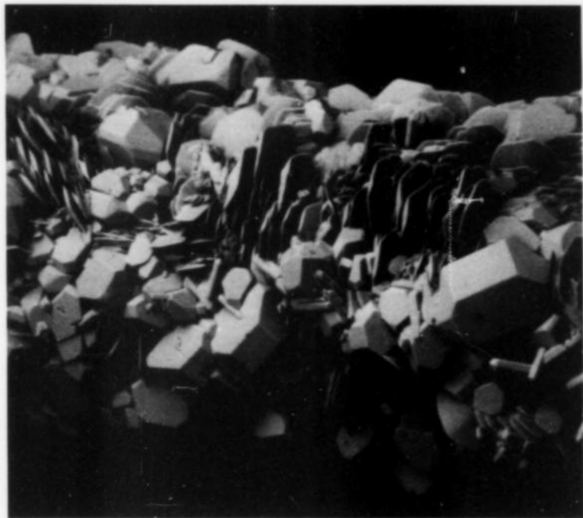
Figure 10. Higher magnification view of Figure 9 showing the complex crystal aggregation of anglesite, bismoclite and quartz. Field of view 0.21 mm x 0.30 mm. G. Dunning specimen and SEM photo.
