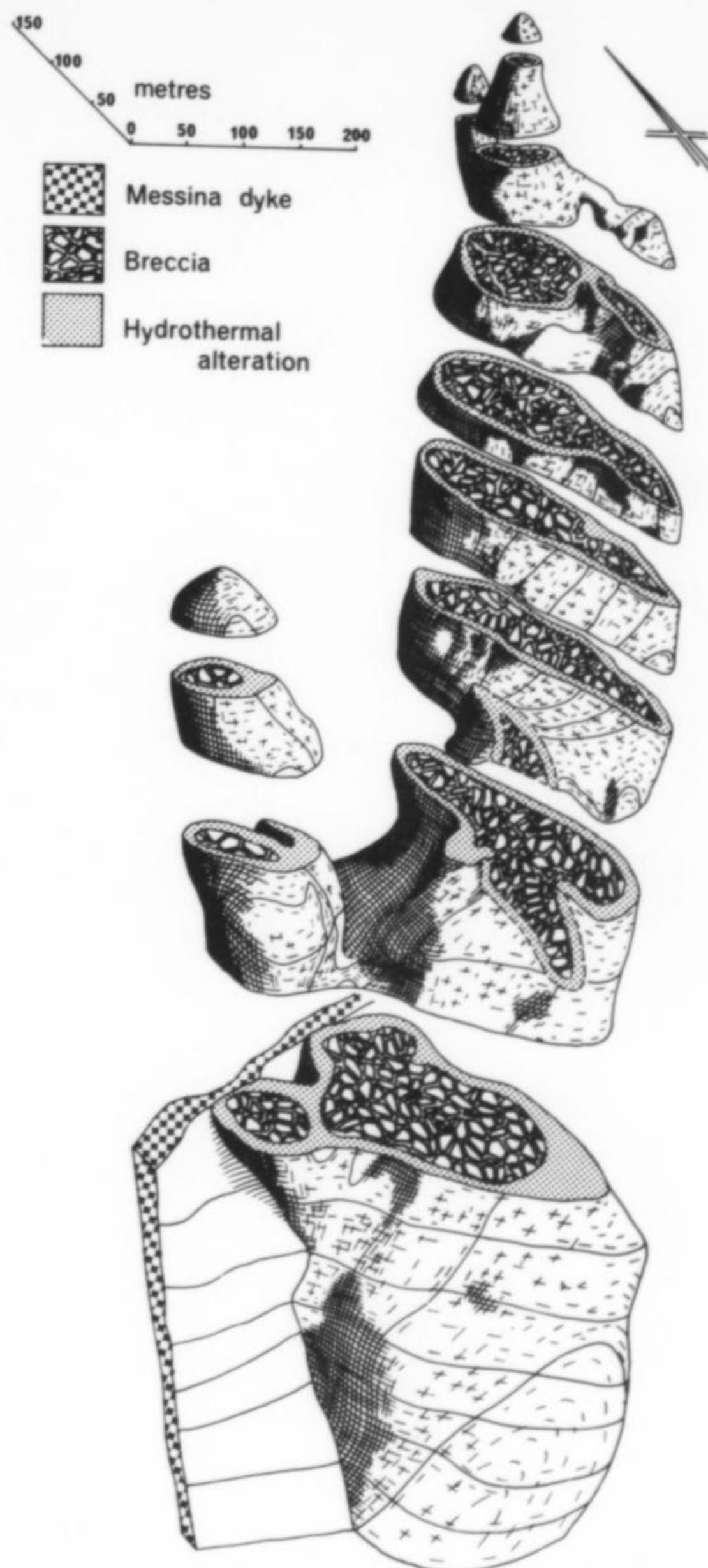
Figure 9. Three-dimensional construction of the L Lode breccia pipe at the Messina mine (from Jacobsen et al. , 1976).
