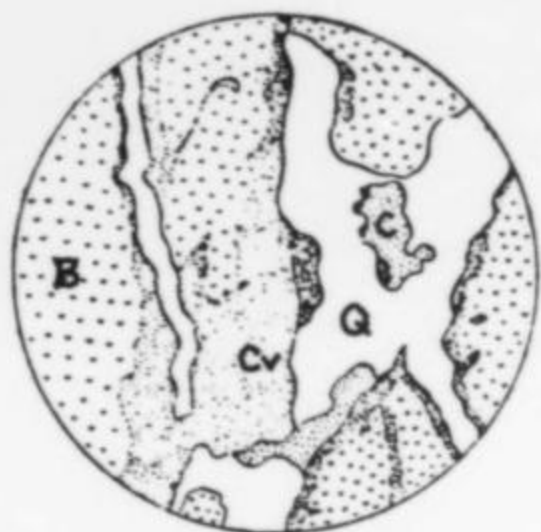
Figure 7a. Sketch of polished surface of benjaminite showing relation of benjaminite to quartz and chalcopryrite and replacement of chalcopryrite and benjaminite by covellite (from Shannon, 1925). Q = Quartz; B = Benjaminite; C = Chalcopryrite; M = Molybdenite; Cv = Covellite.
