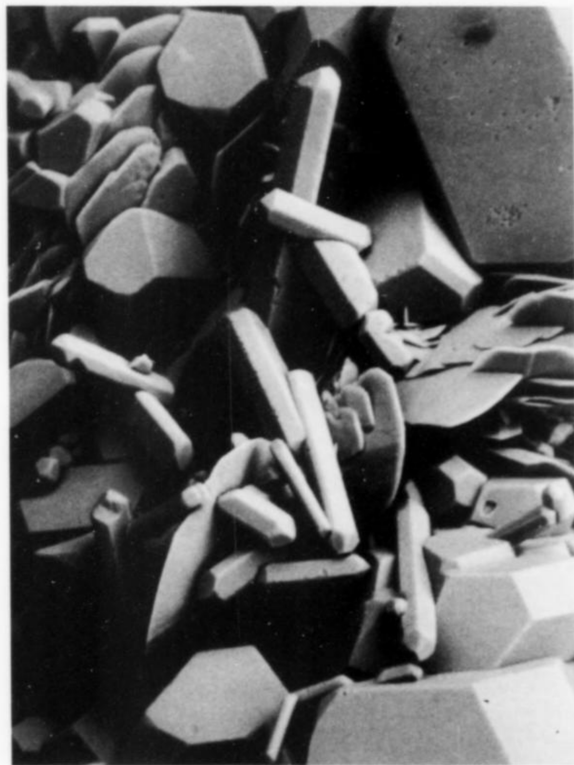
Figure 12. Higher magnification view of Figure 9 showing the individual habits of anglesite, bismoclite and quartz. All of the crystals are transparent and glassy. Field of view is 0.08 x 0.1 mm. G. Dunning specimen and SEM photo.
