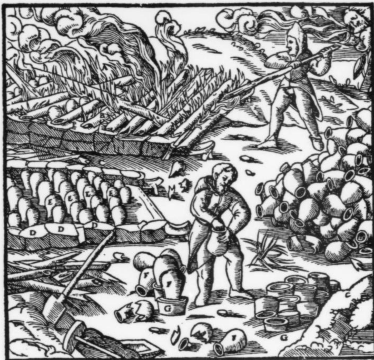
Figure 14. The process of roasting cinnabar to produce metallic mercury (from Agricola, 1556).
