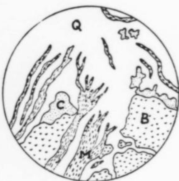
Figure 7c. Sketch of polished surface showing relations of benjaminite, molybdenite, chalcopryrite and quartz (from Shannon, 1925).
