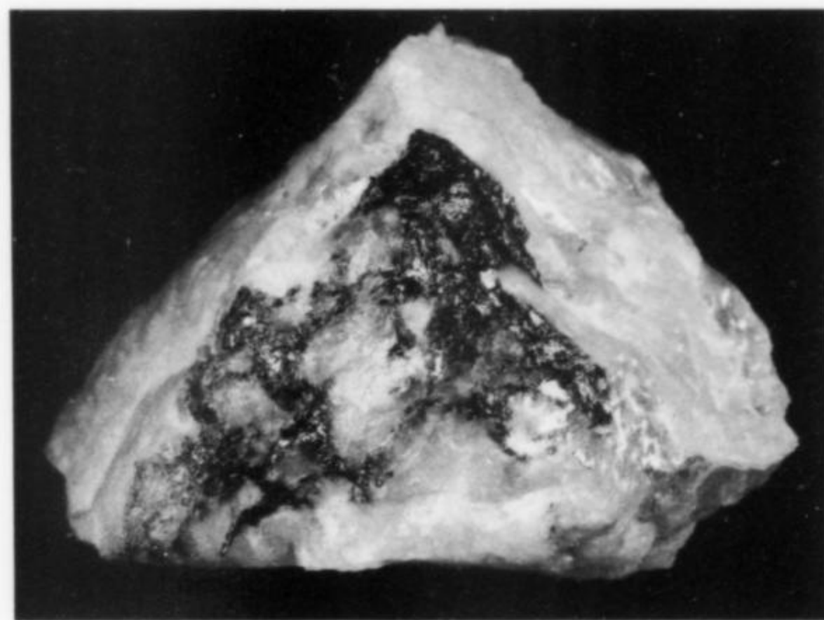
Figure 8. Typical vein quartz sample, 5 x 8 cm, containing metallic seams and pods of aikinite/benjaminite. G. Dunning sample and photo.
