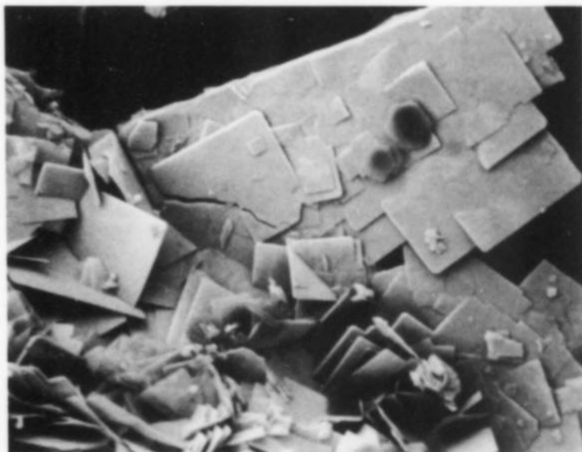
Figure 13. Complex aggregation of bismoclite crystals found lining quartz cavities where the sulfosalts have been oxidized. Field of view is 0.06 x 0.08 mm. F. Cooper specimen and G. Dunning SEM photo.
