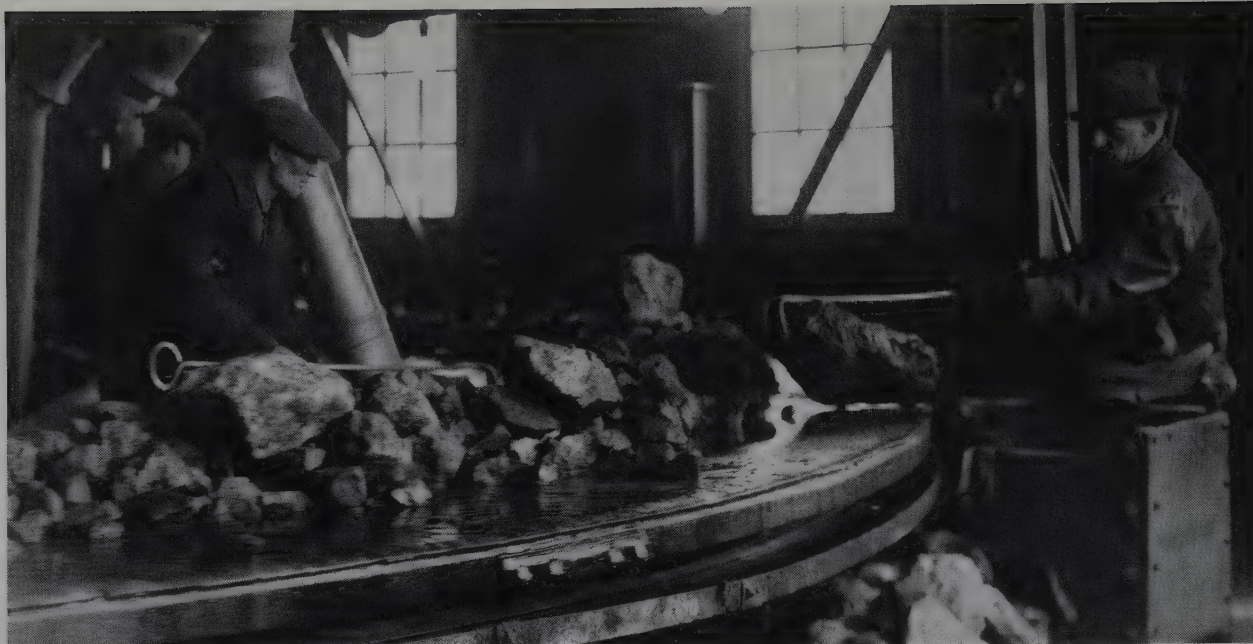
The “picking table” at Franklin, New Jersey (ca. 1945), where low-grade ore, timber fragments and tramp steel were culled out. Photo: Robert Svecz.
