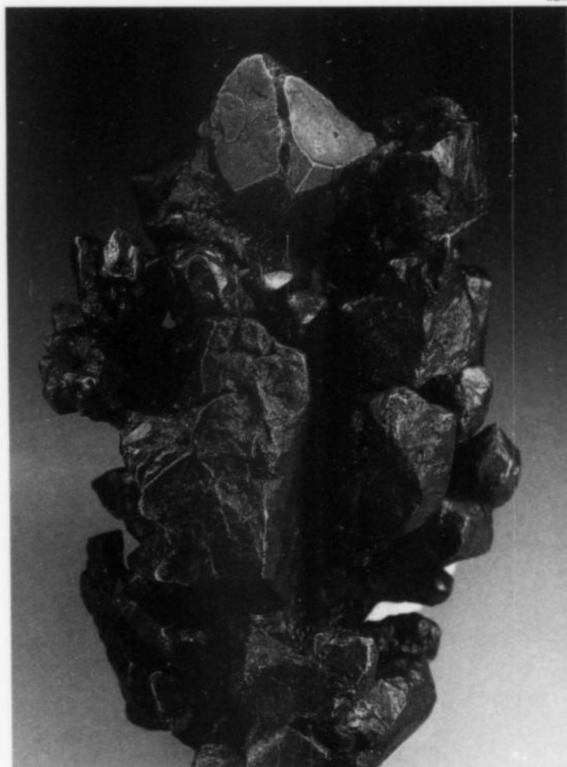
Figure 50. Copper crystal group, 5.4 cm tall, showing rare octahedron modified by hexoctahedron, from Houghton County. Richard Kosnar collection, ex B. S. Butler collection.
