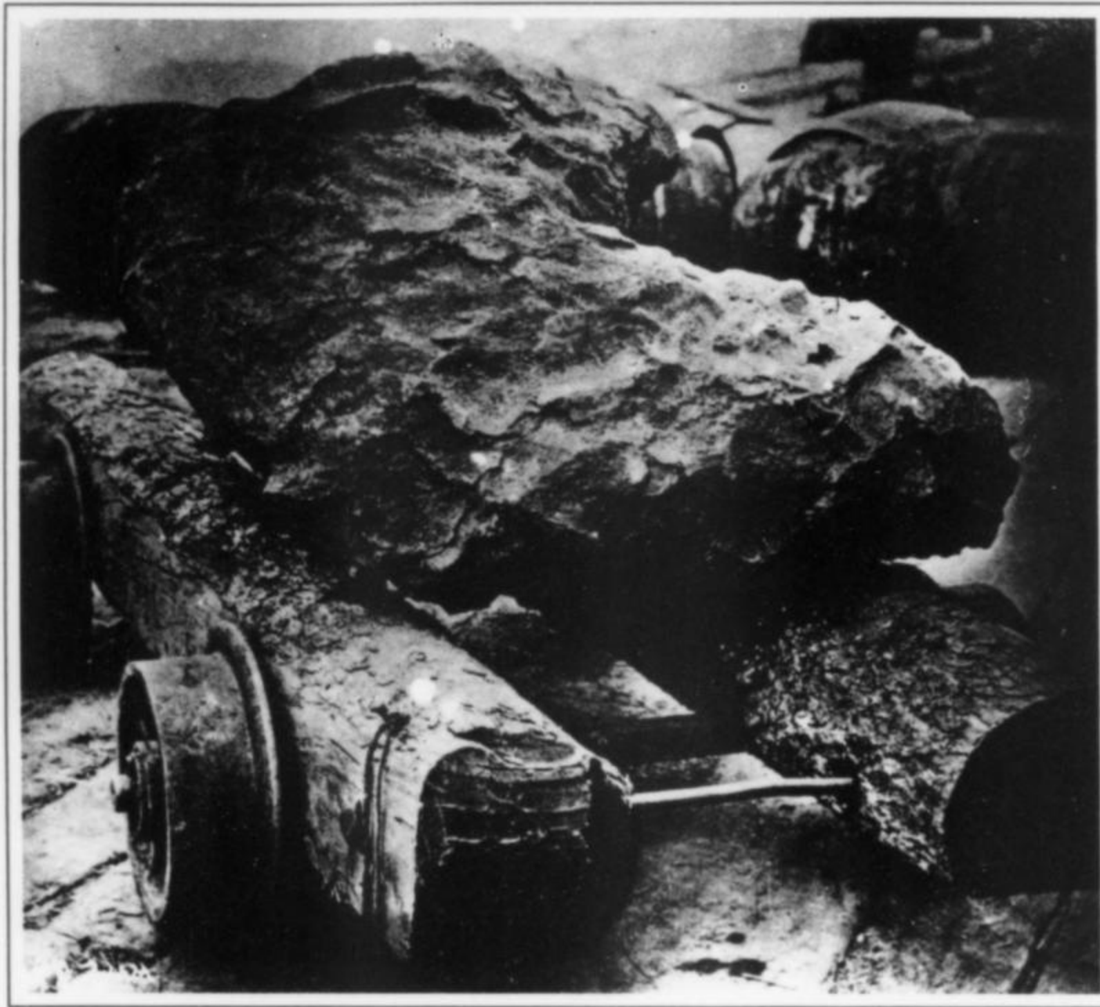
Figure 14. A 6000-pound mass of copper found in ancient Indian workings, in a pit 16.5 feet deep at McCargo Cove on Isle Royale. The marks of crude stone hammers cover its surface. (MTU Archives)
