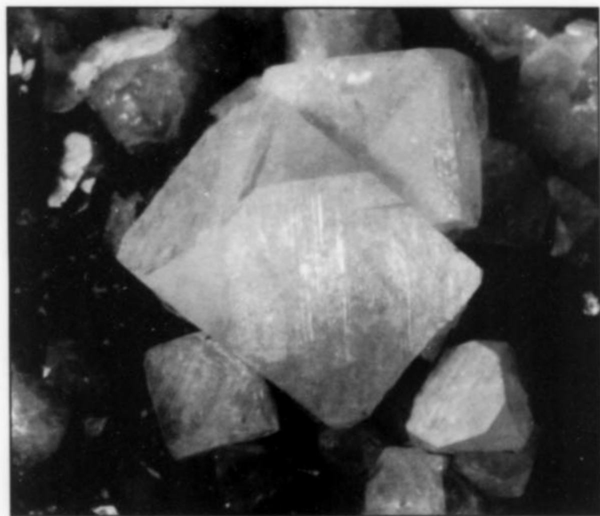
Figure 39. Goyazite crystals, white, to 6 mm, showing the forms r\{10\bar{1}2\} and e\{01\bar{1}1\} , from Area B, locality 10. CMN specimen 50822; G. Robinson photo.
