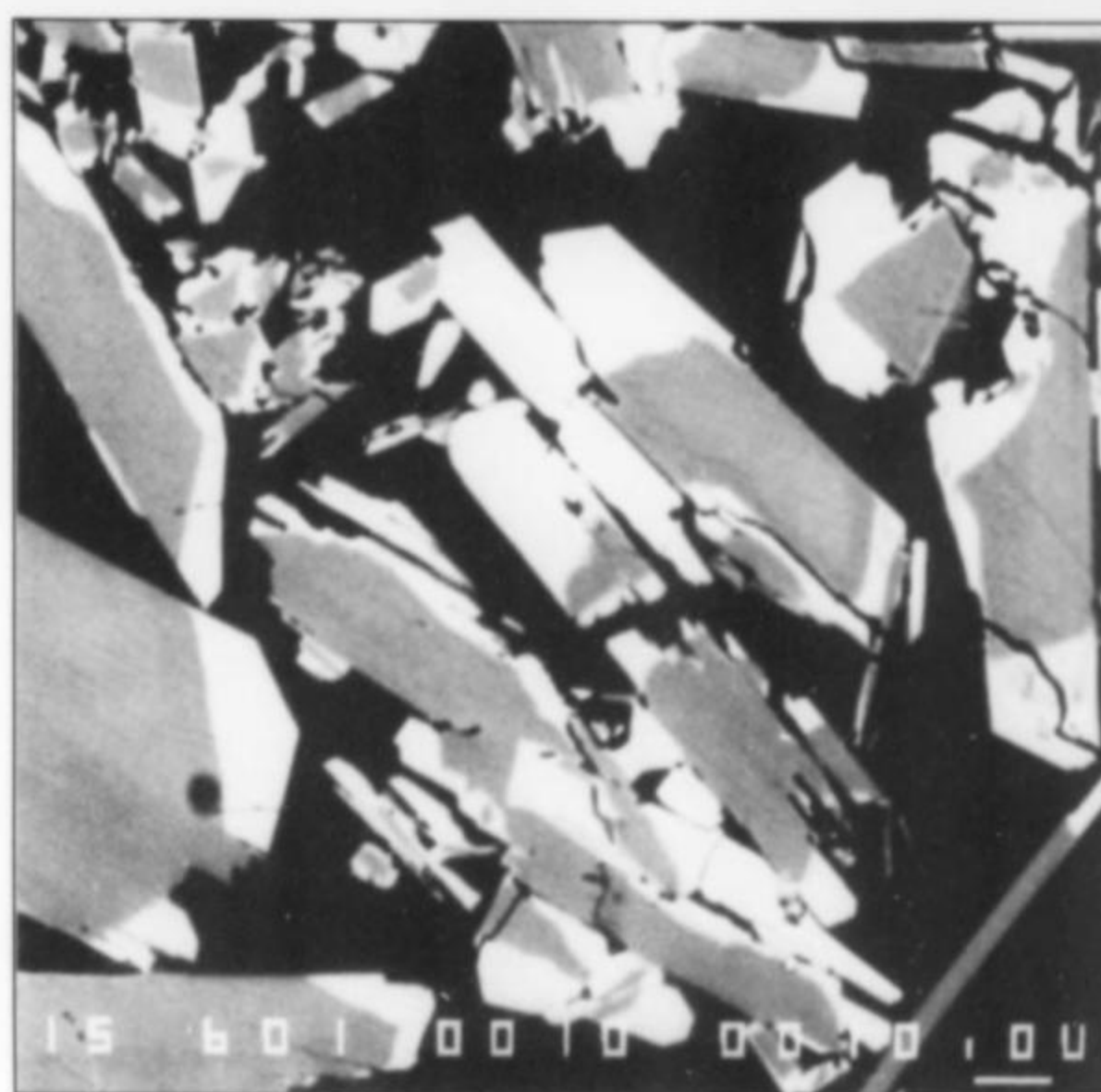
Figure 14. Back-scattered electron image of arrojadite (gray) and the barium analog of arrojadite (white).
