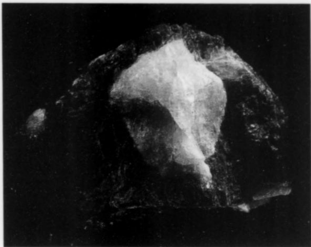
Figure 47. Considerably rarer than cryolite is cryolithionite, with \text{Li}_3\text{Na}_3 rather than \text{Na}_6 in the formula. It is always found completely enclosed in cryolite, and is most easily spotted when (as here) it is in the black variety of cryolite. Size of the specimen, 10 cm; photo by R. Bode.
