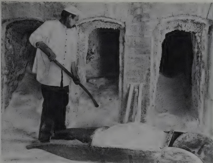
Figure 9. Worker loading a wheelbarrow with arsenic crystals at Tolvadden, Cornwall, 1890. Note cotton swabs in worker's nose for protection against deadly dust. Collection of the Royal County Museum of Truro.
