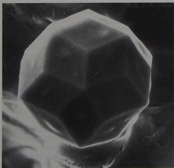
Figure 1. SEM photo of an isolated, triacontahedral quasicrystal of Al_{5.1}Li_3Cu made at AT&T Bell Laboratories. The grain is 0.1 mm across. SEM photo courtesy of A. R. Kortan, AT&T Bell Laboratories.
