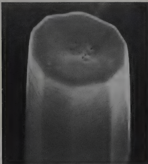
Figure 16. (a) SEM photo of decagonal grains of Al-Cu-Co which are approximately 0.07 mm across. (b) Enlargement of the decagonal grain in the center of (a). Courtesy of A. R. Kortan, AT&T Bell Laboratories.
