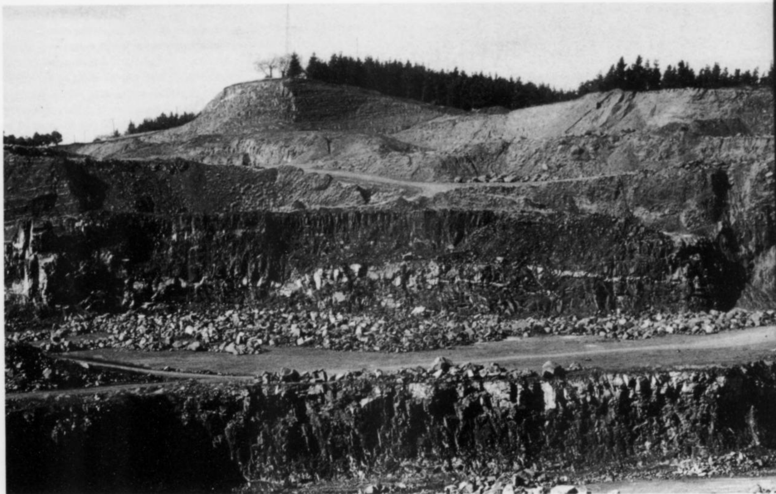
Figure 1. Panoramic view of the eastern face of Prospect quarry in October of 1981. The dark chilled basalt margin and pegmatite/microdolerite schlieren are clearly visible. Lower level of the quarry is in picrite. Photograph by the author.
