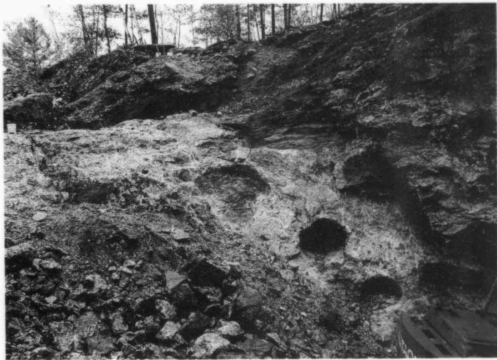
Figure 3. Excavated beryl-bearing pockets in the cleavelandite replacement unit along the north wall of the quarry.
