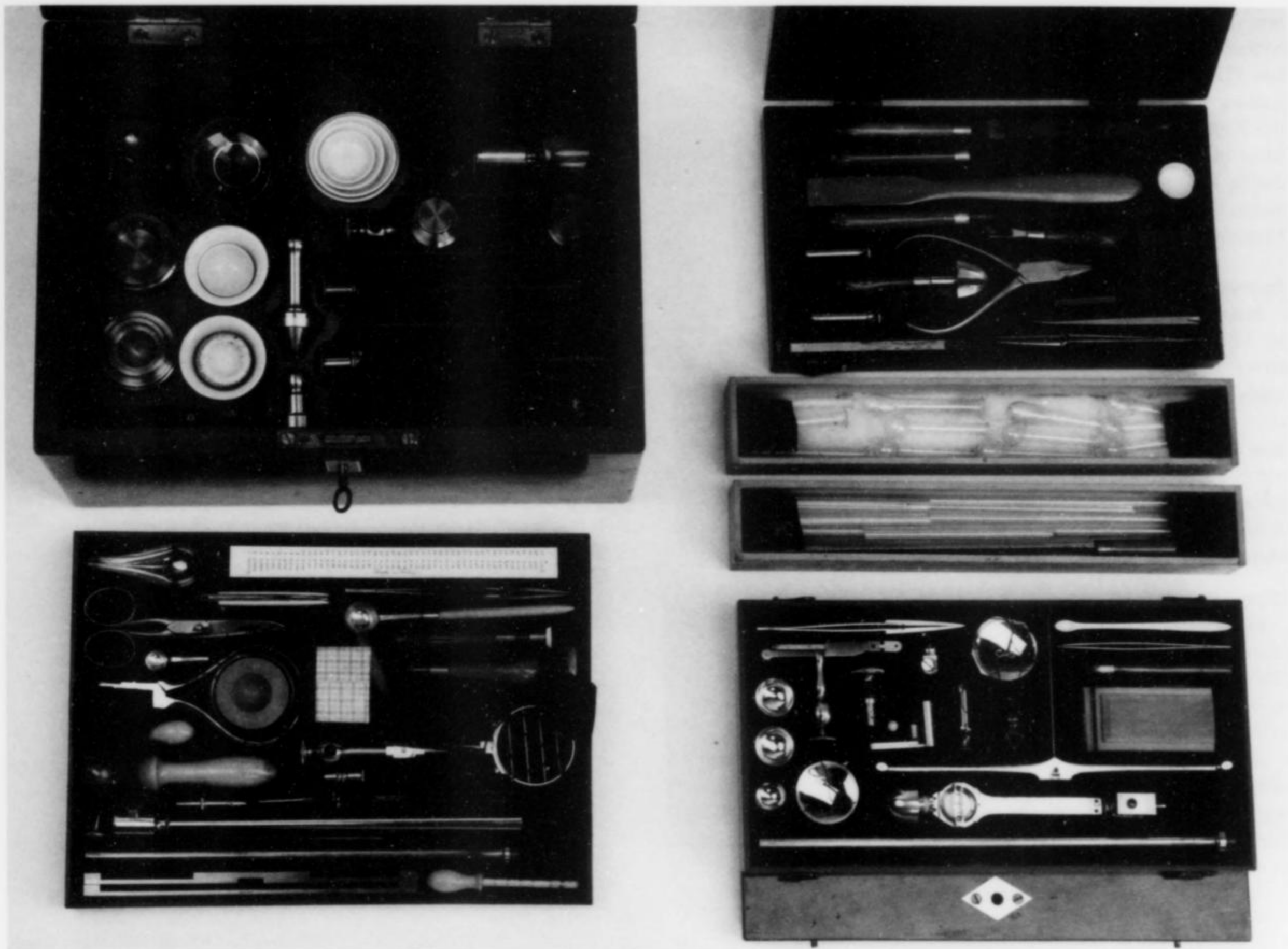
Figure 24. Trays of blowpipe utensils in the Freiberg Apparatus made by Lingke, Freiberg, ca. 1870.
