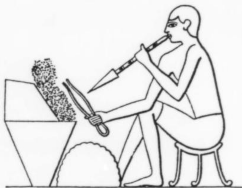
Figure 1. Illustration of an Egyptian silversmith with a blowpipe; Theba, circa 1500 B.C. (Haughton, 1862).
