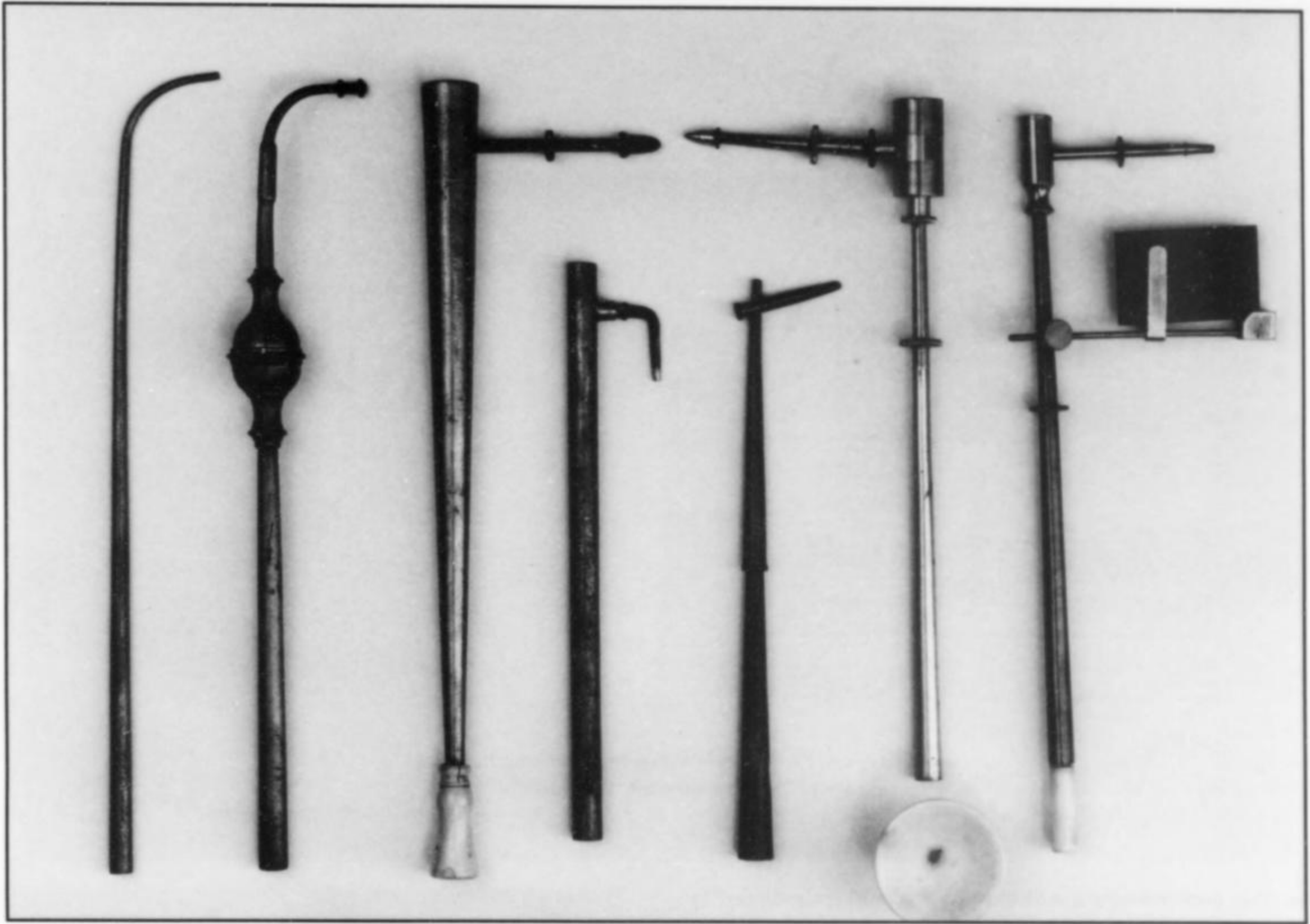
Figure 10. Blowpipe types (left to right): simple, Cronstedt, Black, Tennant, Wollaston, Gahn, Hirschwald with cobalt-glass.
