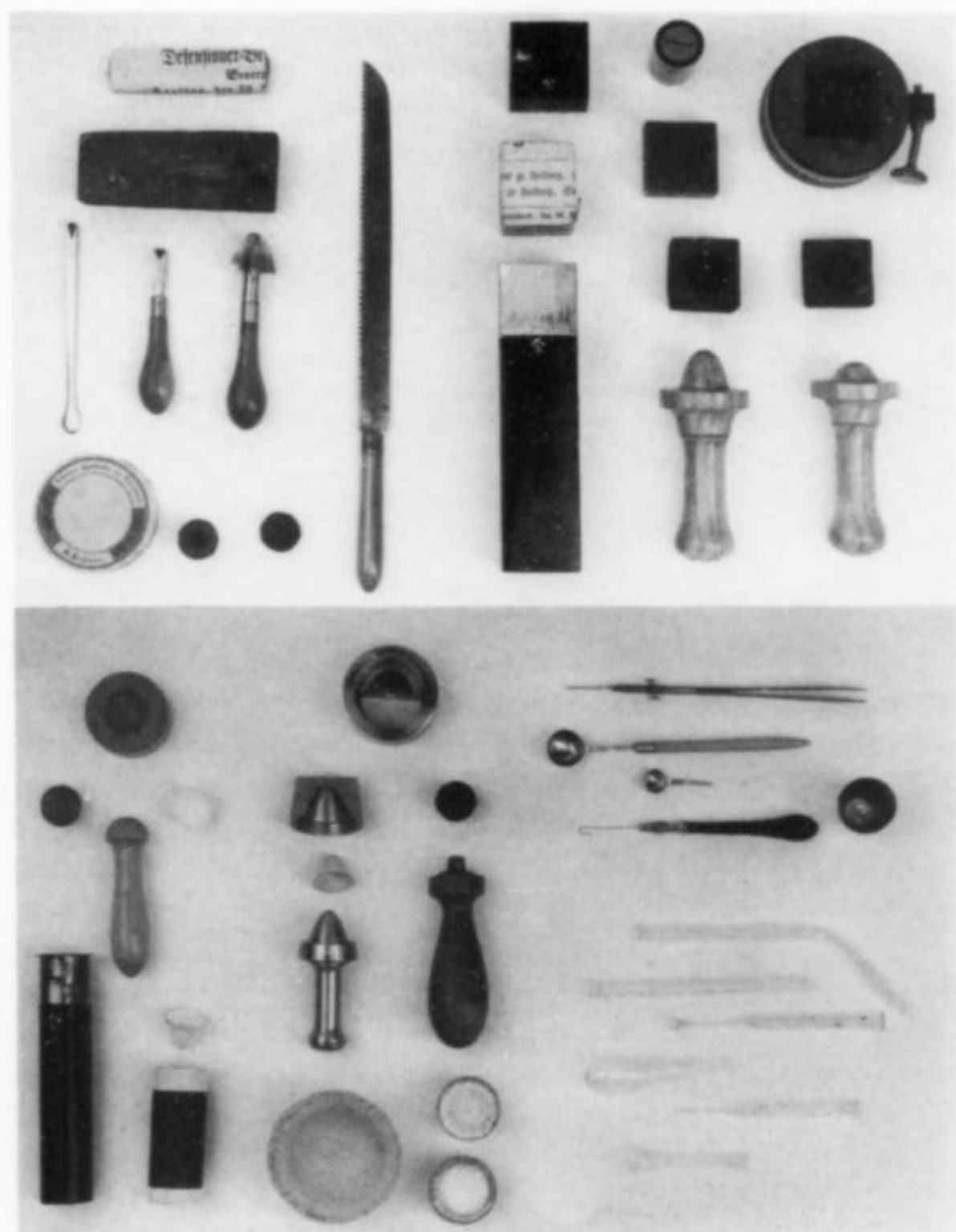
Figure 15. (Top:) Charcoal supports and tools used in blowpipe analysis. (Bottom:) Clay, platinum and glass supports used in blowpipe analysis, with molds for making crucibles.
