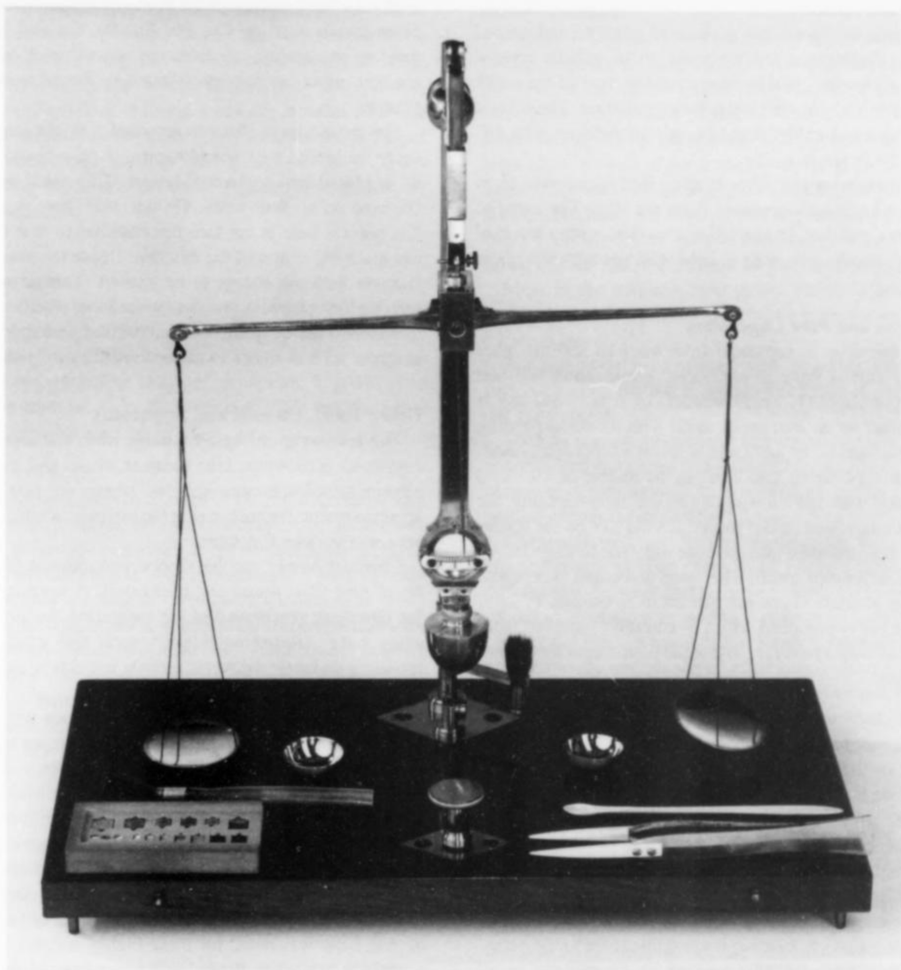
Figure 17. Collapsible analytical balance, ca. 1870, by Lingke of Freiberg.
