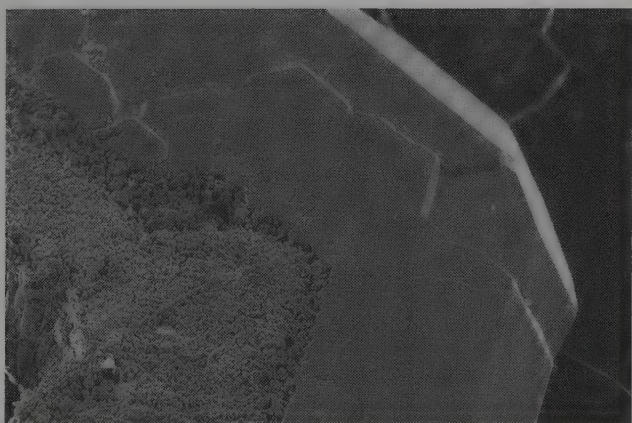
Figure 9. SEM photograph of the edge of a composite niobian rutile-hematite crystal showing the perfection of growth of the hematite relative to the multiple nucleation growth of the niobian rutile.
