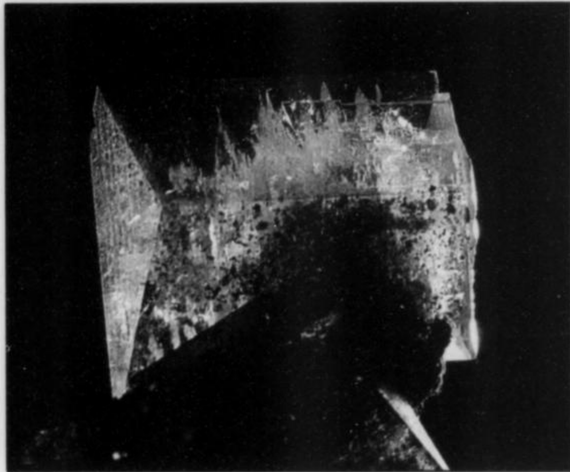
Figure 11. Single hyalophane crystal, 1.7 cm, elongated in the direction of the b -axis. Cleavages along (001) can be seen, as well as hematite inclusions. M. Žorž specimen and photo.
