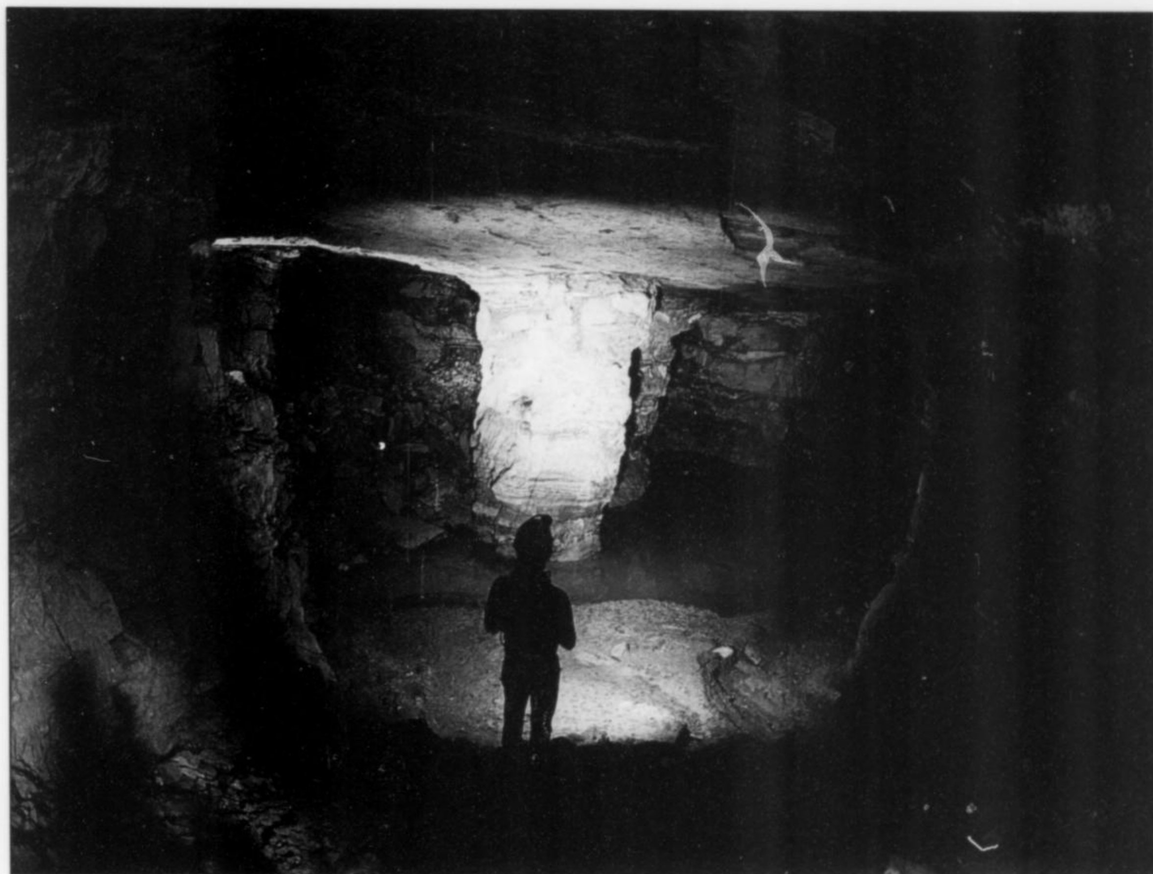
Figure 31. Room and pillar mining at the Victory mine, typical of the way bedding-replacement deposits near Cave in Rock were mined. Chris Anderson photo.
