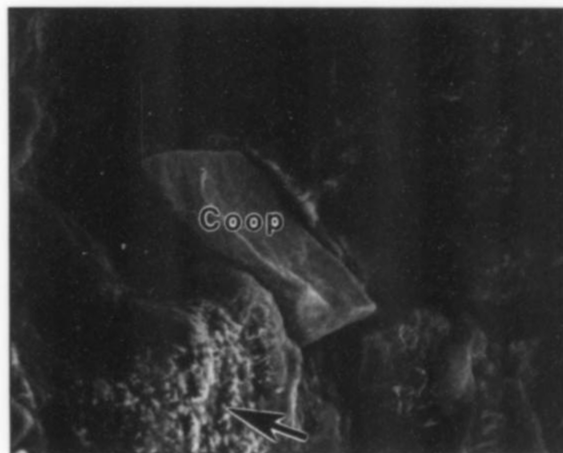
Figure 4. Secondary electron image showing a 30-micron grain of cooperite (Coop), Pt-Cu and amorphous siliceous mixture intergrowth (arrow) which line a cavity in the ferroan platinum crystal.
