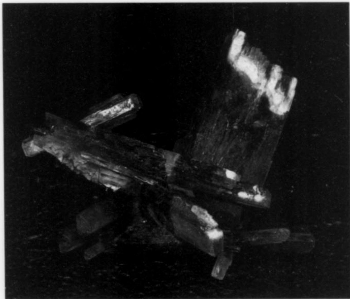
Figure 5. Barite crystal group; 13.8 cm long; from Stoneham, Weld County, Colorado (after treatment). The larger epoxy restoration is clearly visible in the center of the front crystal.
