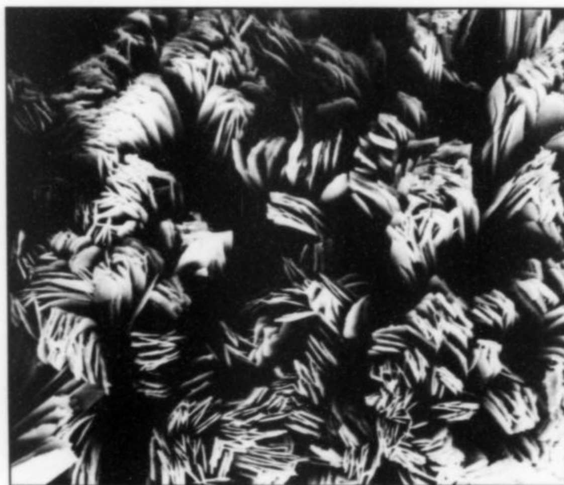
Figure 2. Scanning electron photomicrograph of sheaves of utahite.
