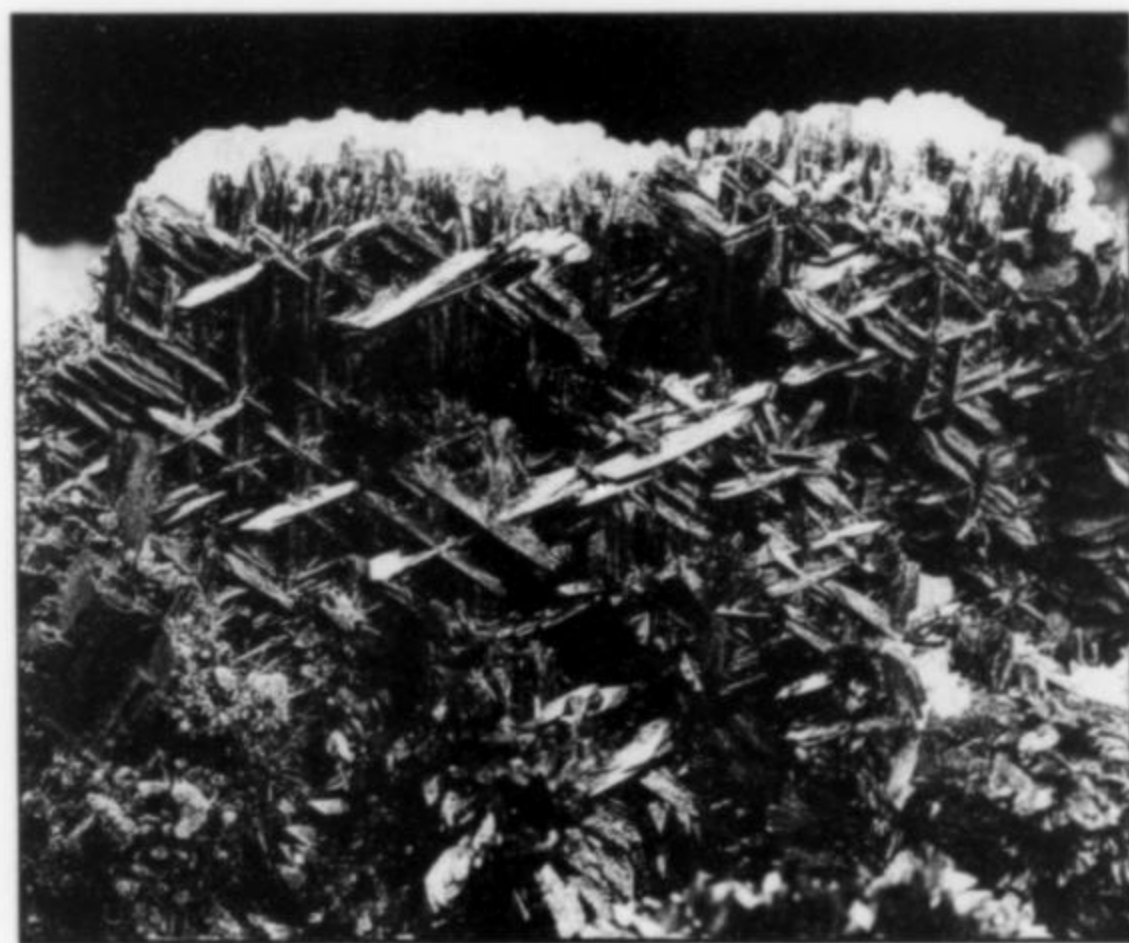
Figure 53. Reticulated arsenopyrite crystals, 3 cm across, from Huanzala. Gene Schlepp collection; Wendell Wilson photo.
