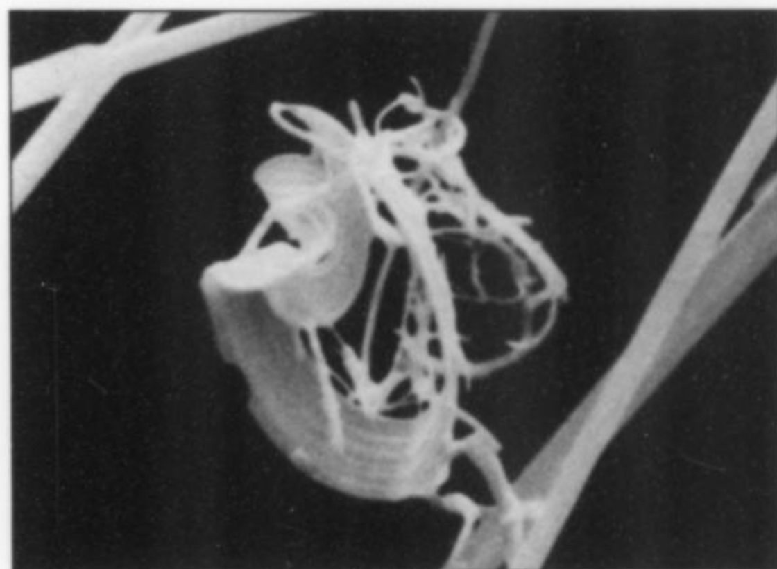
Figure 33. Rings and curls, 0.004 mm across, of an unknown Ni-sulfate. Rudi Turner specimen and SEM.
