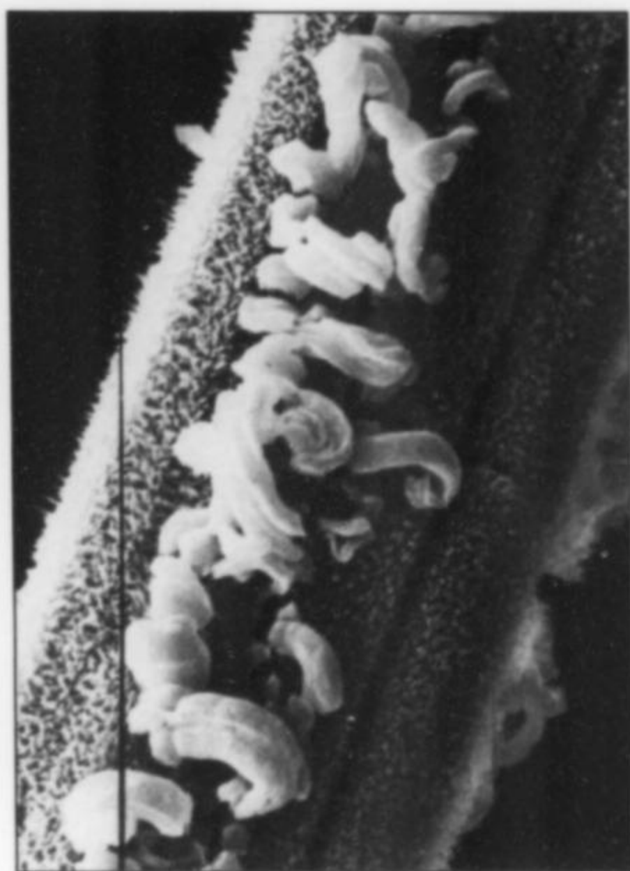
Figure 15. Millerite needles, 0.01 to 0.03 mm across, altering to vermicular or ram's-horn jamborite (?). Rudi Turner specimen and SEM.
