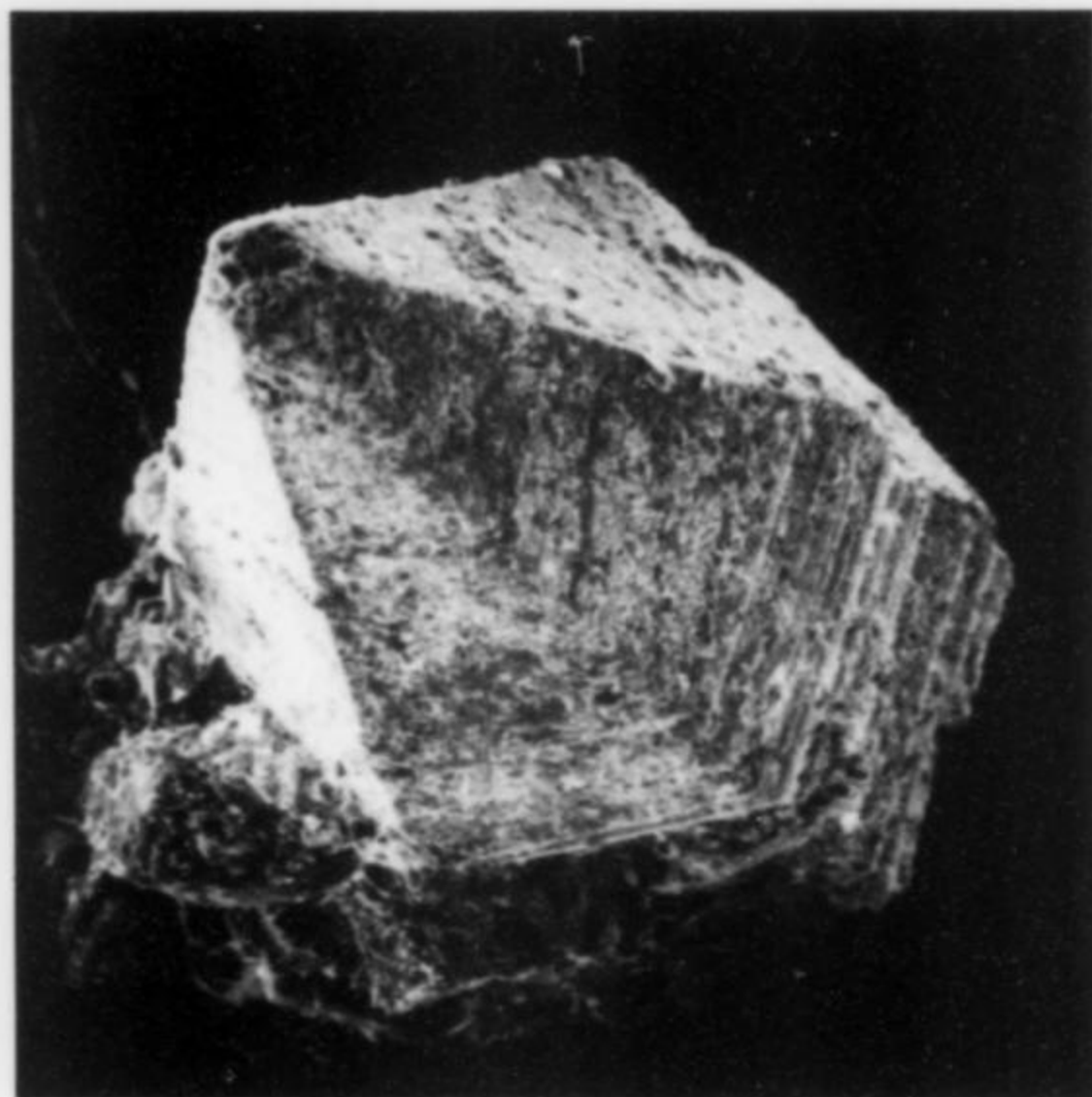
Figure 2. Scanning electron microscope image showing the hexagonal dipyramid termination of a pseudomorph. Note the characteristic striations perpendicular to the c-axis on the "prism" faces. These striations can be used to distinguish paralstonite from calcite.
