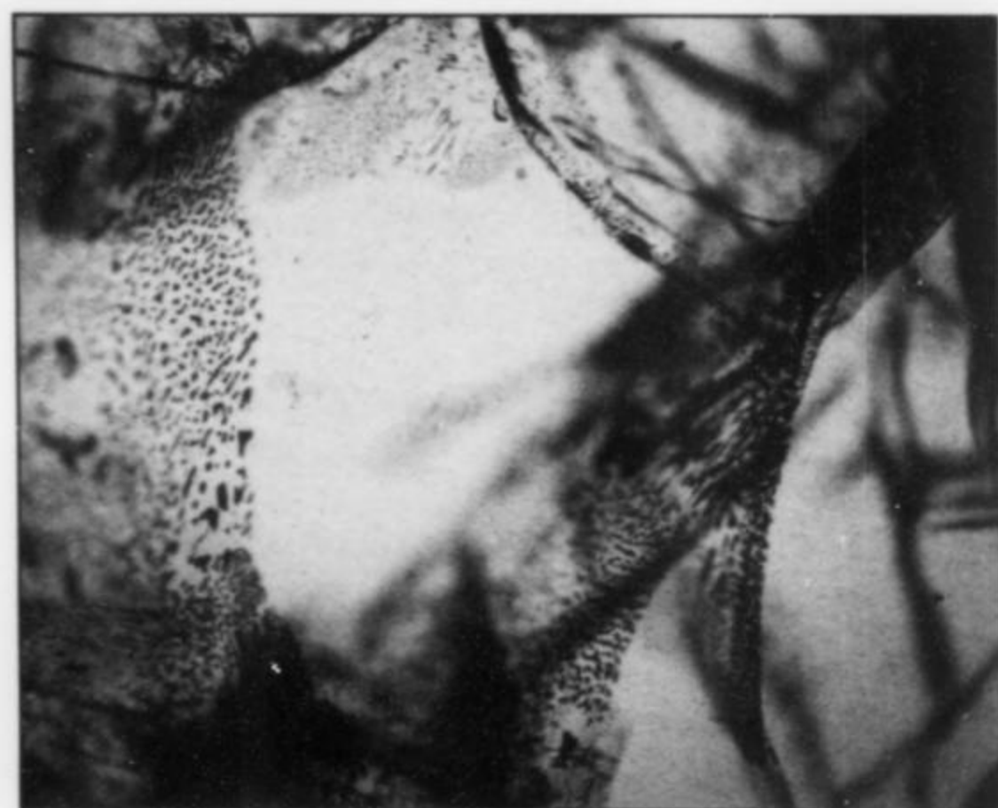
Figure 8. Fingerprint-like inclusion layers resulting from fracture healing in eosphorite (30X).
