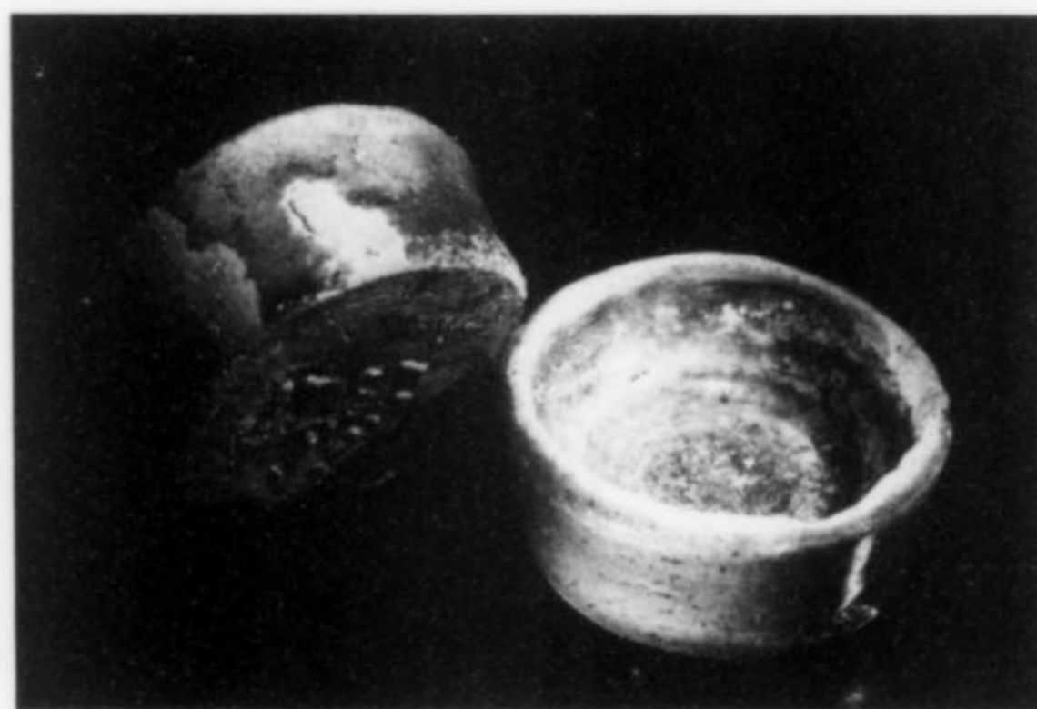
Figure 2. Old silver-smelting or assaying cupels from the Annaberg district, ca. 1782. Collection and photo: Peter Huber.
