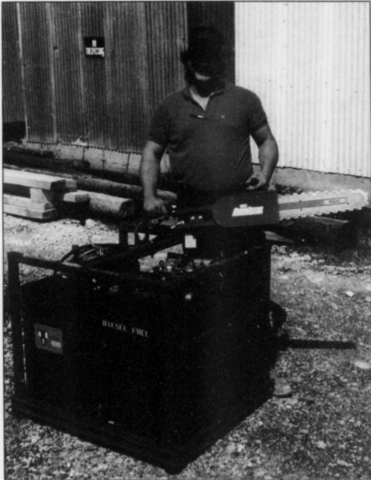
Figure 74. Roger Stiner displays the Sweet Home mine's new diamond chainsaw. Due to this recently developed device, many great rhodochrosite specimens are being preserved. Photo by Bryan Lees.
