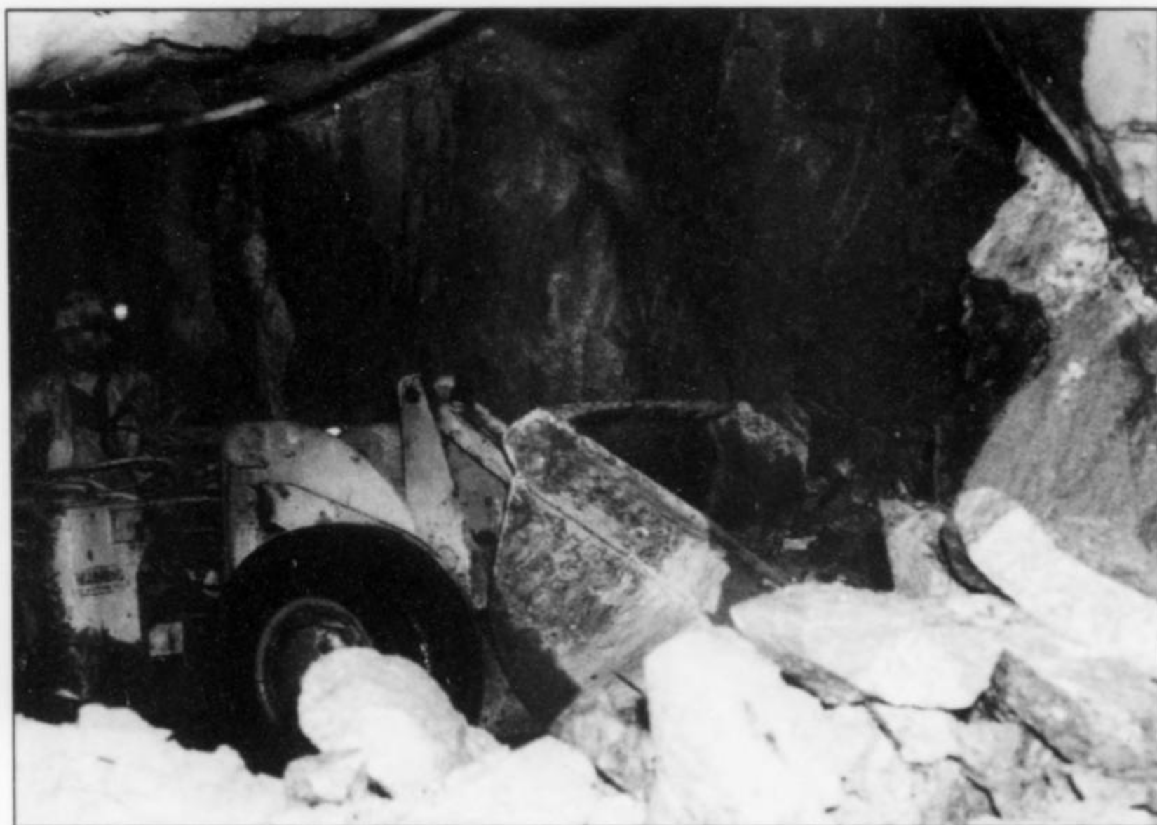
Figure 106. Rodney Orten uses an LHD (Load Haul Dump) to remove blast rock from the bottom of the Main Stope in 1995. Photo by Bob Jones.
