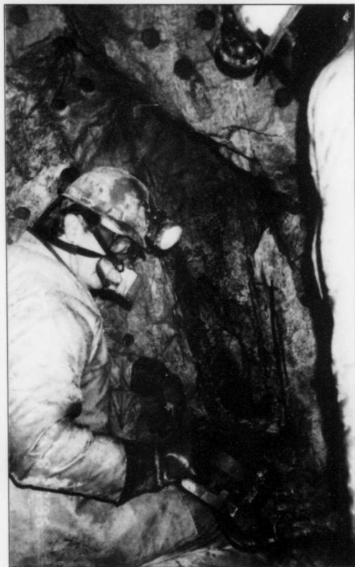
Figure 125. Bryan Lees ( left ) uses a diamond chainsaw to peel rhodochrosite plates out of the Hedgehog Pocket. Photo by Albert Lees.
