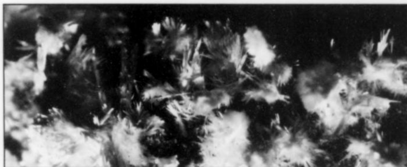
Figure 12. Sprays of munitrite crystals in a cavity from slag material from the Highveld Steel and Vanadium Corporation processing plant. Field of view is 7.2 mm. Windisch specimen M28/1; Cairncross photo.
