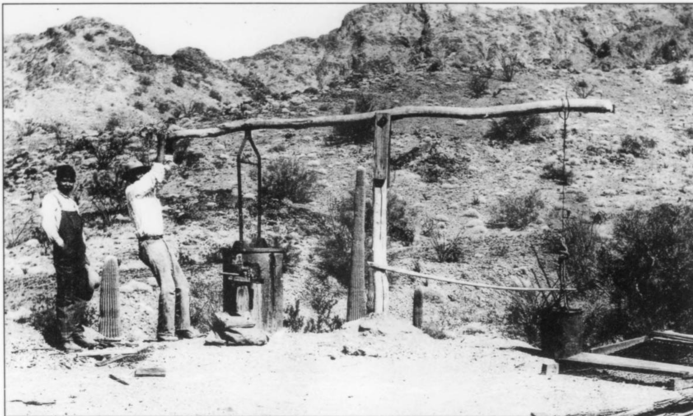
Figure 7. A primitive Mexican-style concentrator in use at Castle Dome in 1919; it could process 50 pounds of ore in 10 minutes. Courtesy Arizona Geological Survey.
