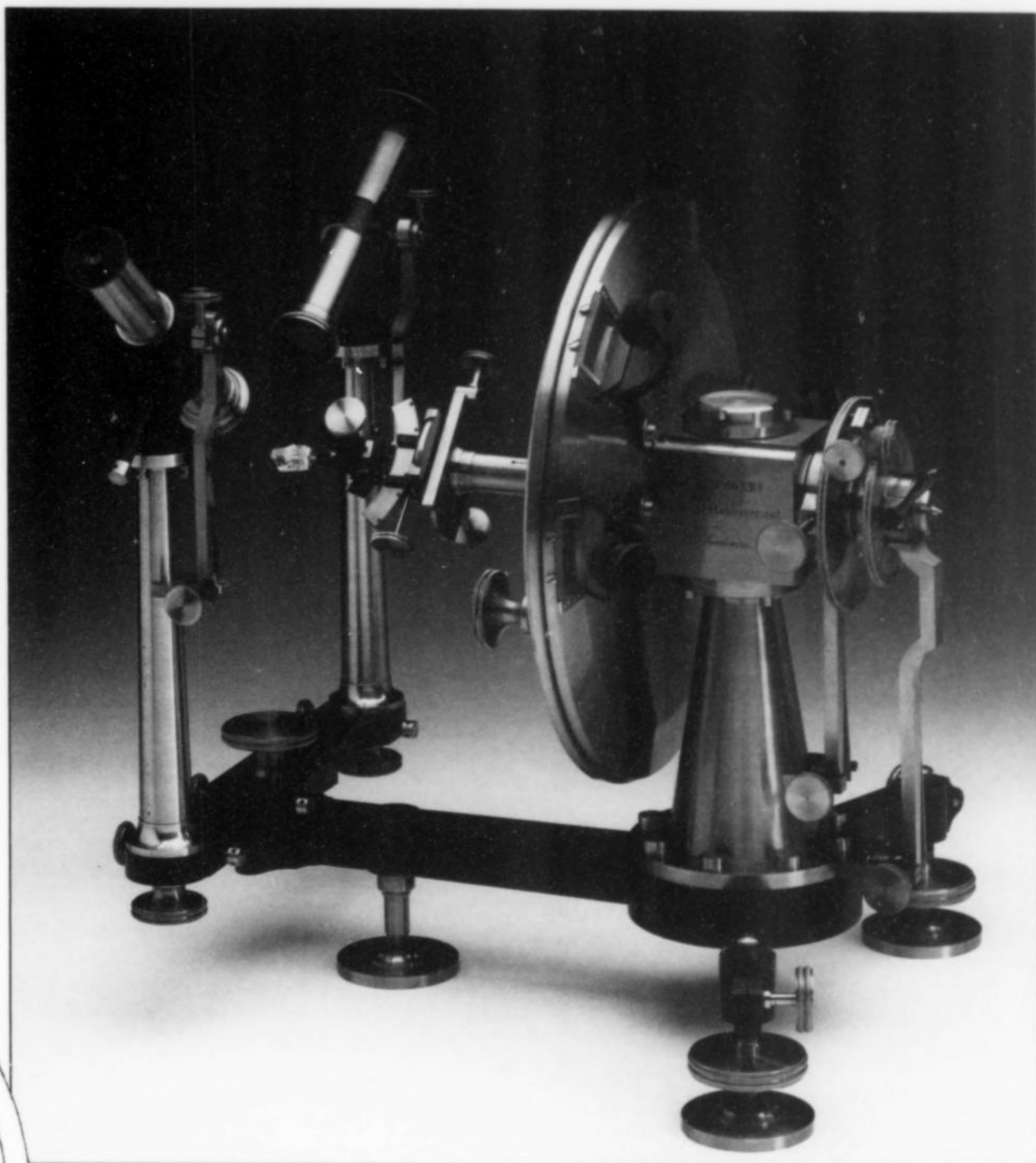
Figure 61. Mitscherlich-type goniometer, signed: "E. Jünger's Mekaniske Etablissement i Kiöbenhavn," purchased in 1878. University of Innsbruck collection.
