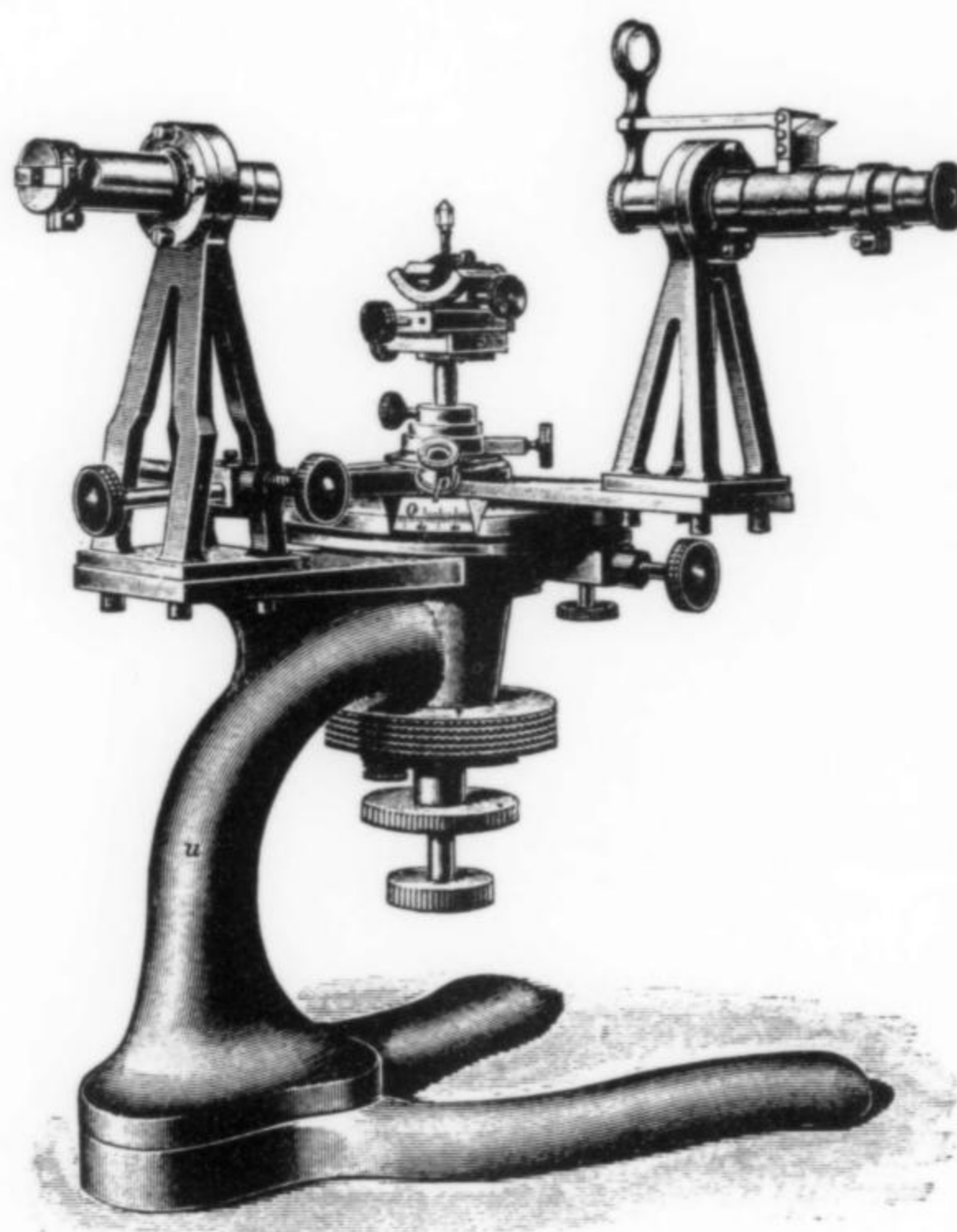
Figure 73. Goniometer by Troughton & Simms, London (Tutton, 1922).
