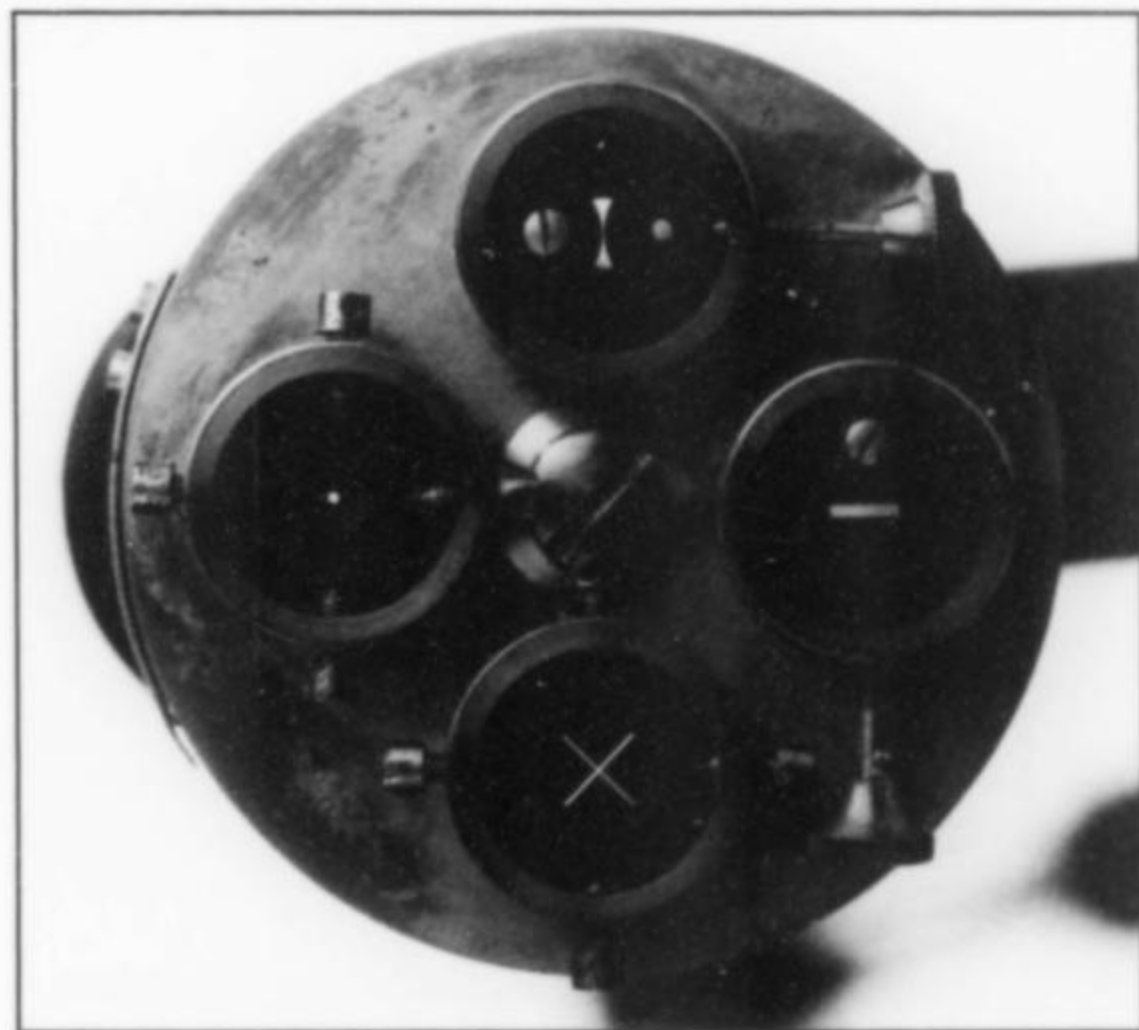
Figure 68. Revolving disc showing the four collimator signals. Clockwise from right: rectangular slit, "Schrauf" signal, round pinhole, "Websky" slit.
