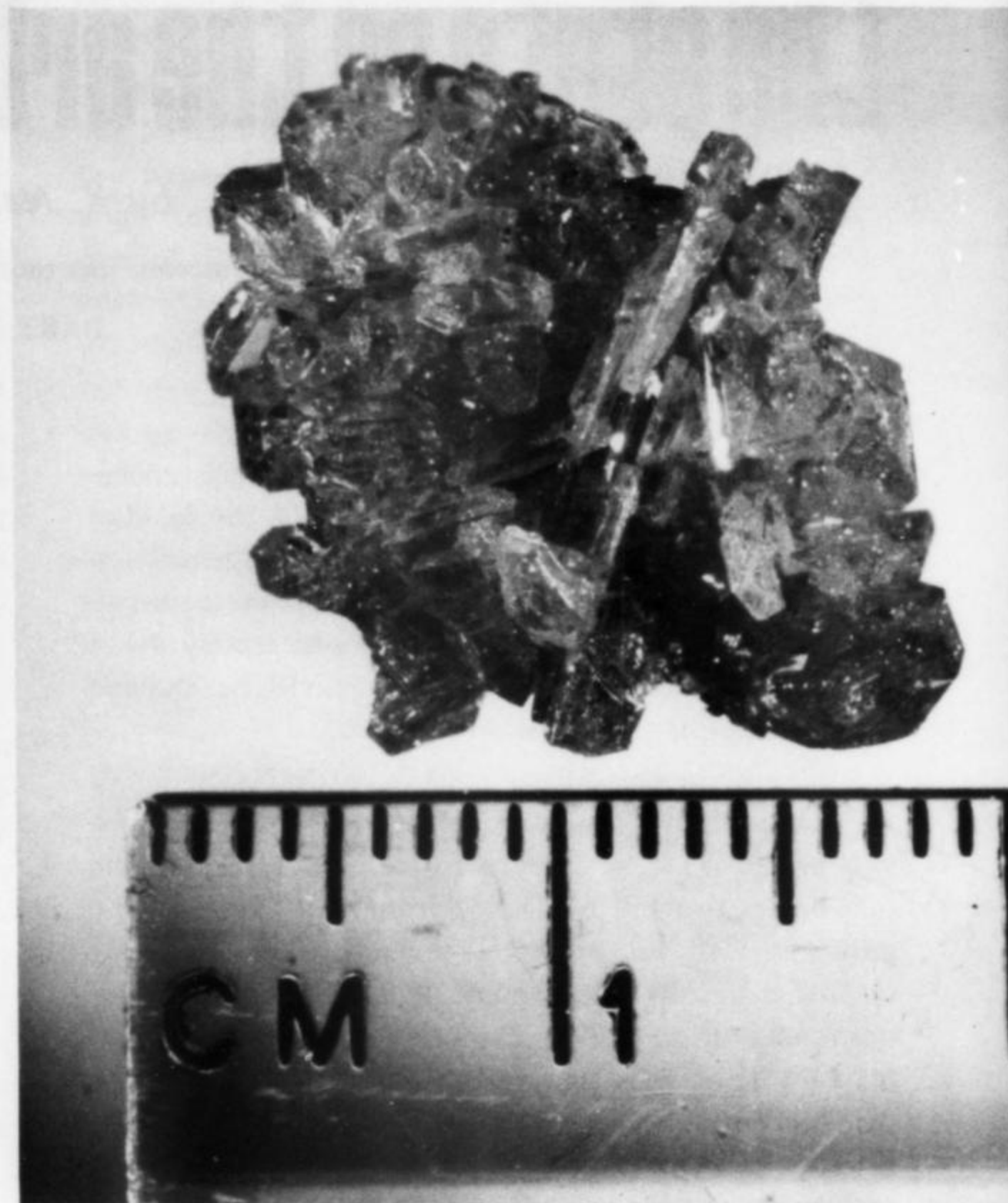
Fig. 3. Hydrothermally grown greenockite.
