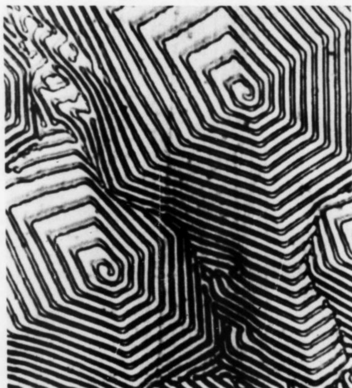
Fig. 9. Growth spirals on a solution grown crystal.
