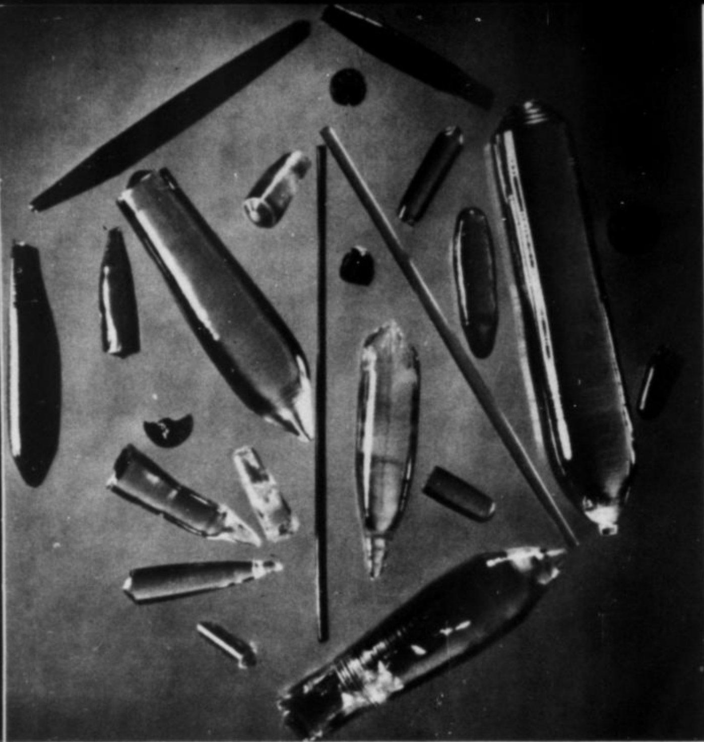
Fig. 1. Czochralski grown scheelite crystals; largest is 6 inches long.
