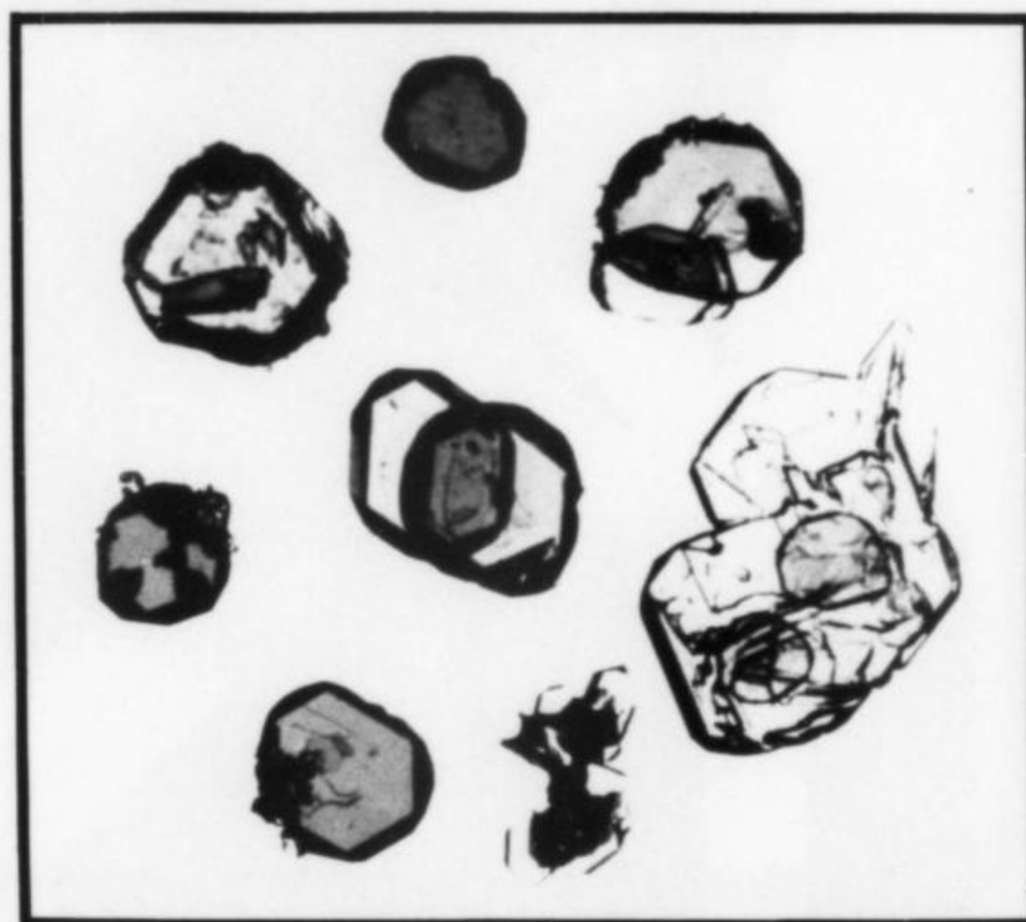
Fig. 5 — Fremy and Verneuil rubies, grown about 1890; largest cluster is 1/4 inch in size.
