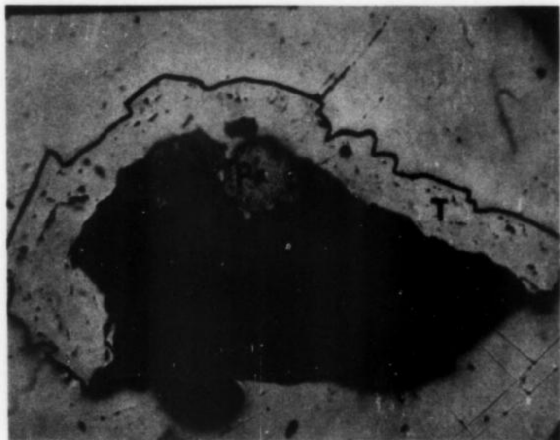
Fig. 5. Polished section showing tennantite-tetrahedrite (T), chalcopyrite (C), and pyrite (P). The tennantite-tetrahedrite shell is approximately 0.5 mm thick. Smithsonian Institution specimen #123091. Photo by Joseph A. Nelen
