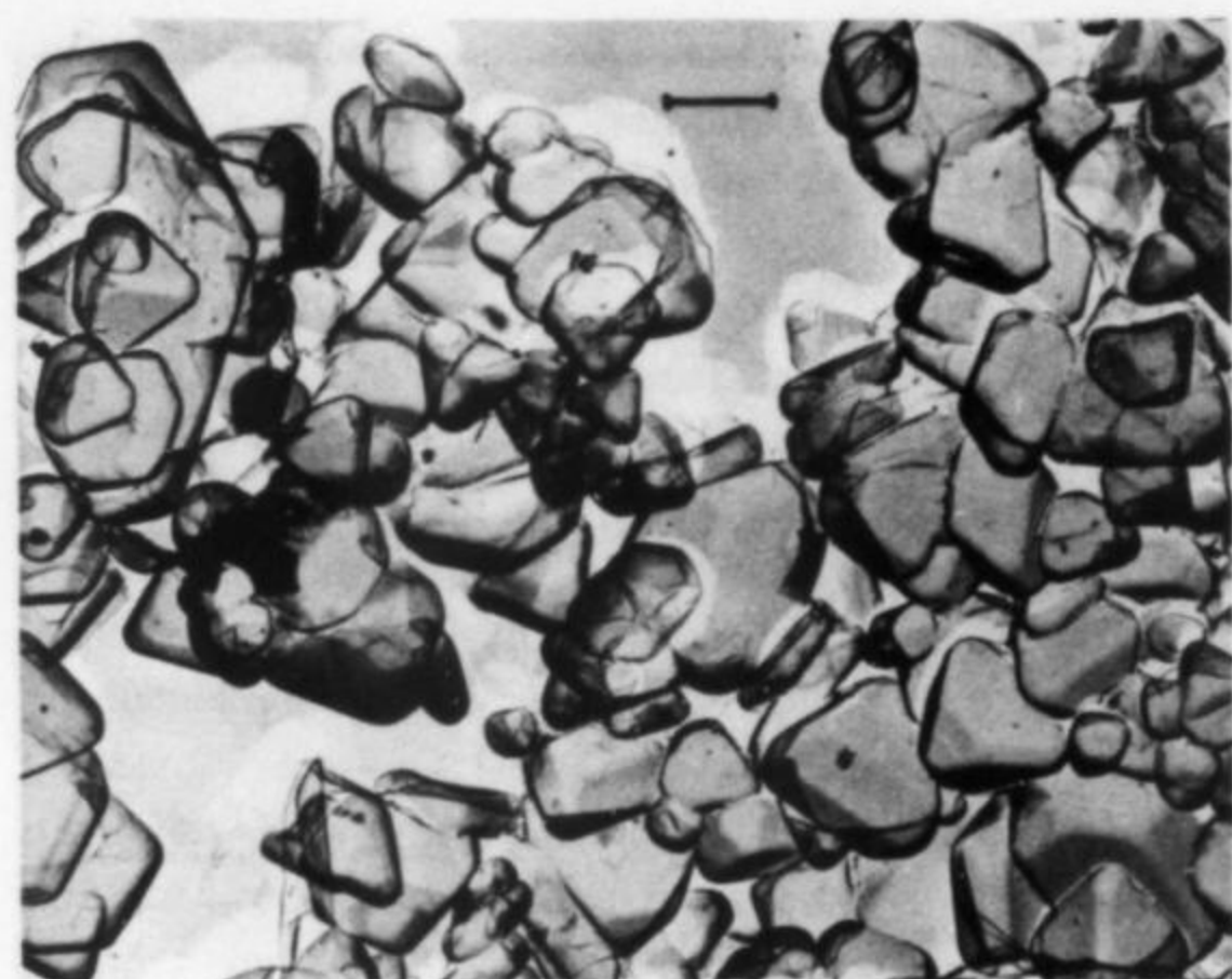
Fig. 6. A transmission electron micrograph of silver bromide crystals (synthetic bromyrite to mineralogists) from the emulsion of a photographic plate. The "replica" technique was used for this picture because electrons are equally as destructive as light would be on the emulsion. The scale bar is 1 micron. Photo courtesy of 3M Company.
