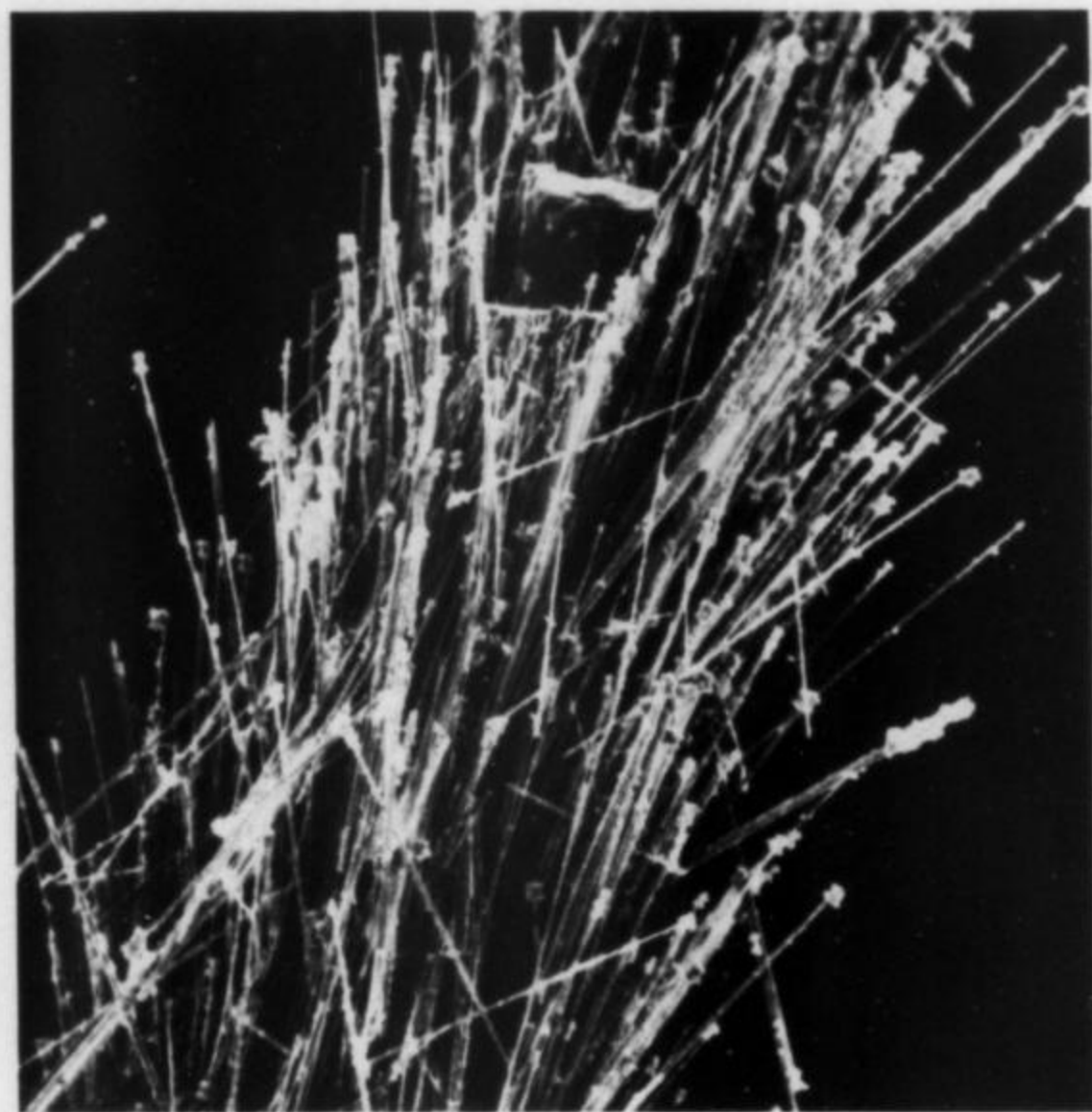
Fig. 9a. Acicular goethite with platy goethite crystals at the end of the needles. X150. NMNH.
