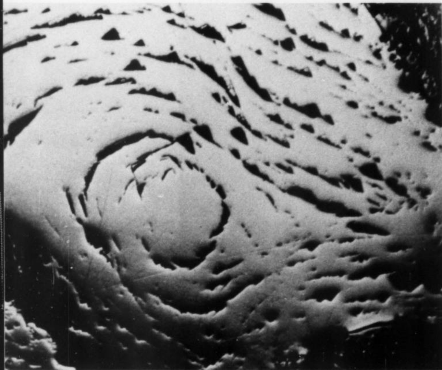
Fig. 7. Deformational characteristics of galena. Note triangular cleavage pits. Photomicrograph by the author. 80X.
