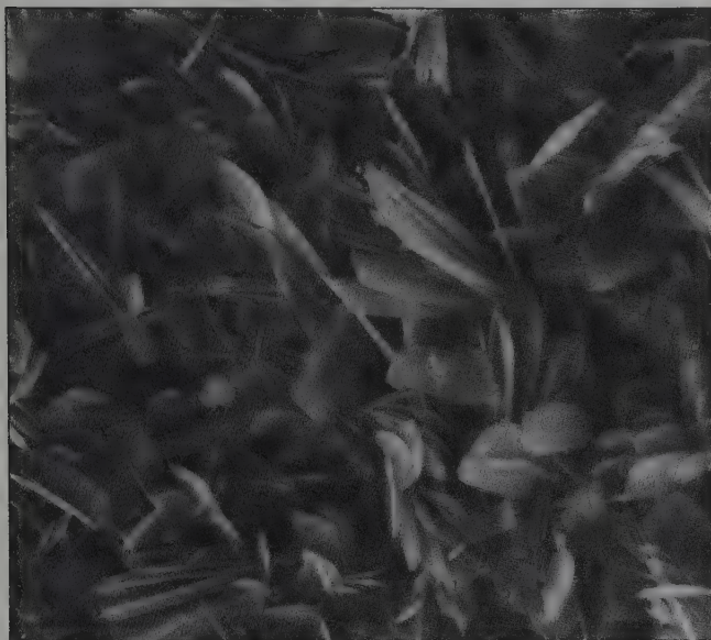
Figure 20. Nb-oxide (hydrated) alteration product of pyrochlore-betafite. SEM photo; crystals are 2 to 8 \mu m.
