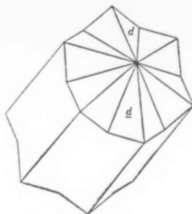
Figure 20. Sal ammoniac crystal drawing taken from Dana's System of Mineralogy (Palache et al. , 1951) showing the dodecahedron twinned on [111] .
