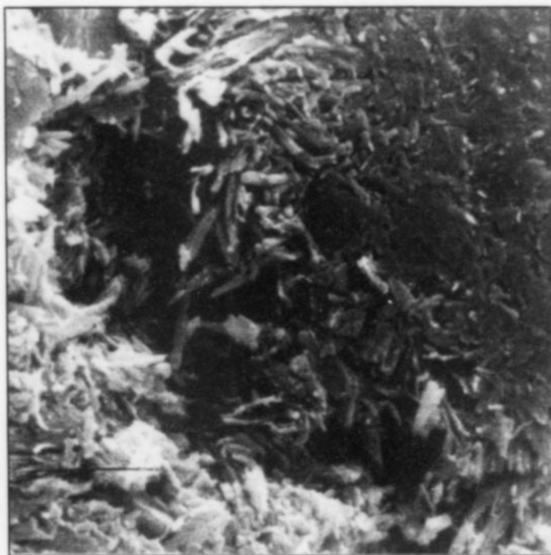
Figure 14. Irregular columnar chapmanite crystals, 2–4 \mu\text{m} long, on rock. Pavel Uher specimen; Ivan Holický SEM.
