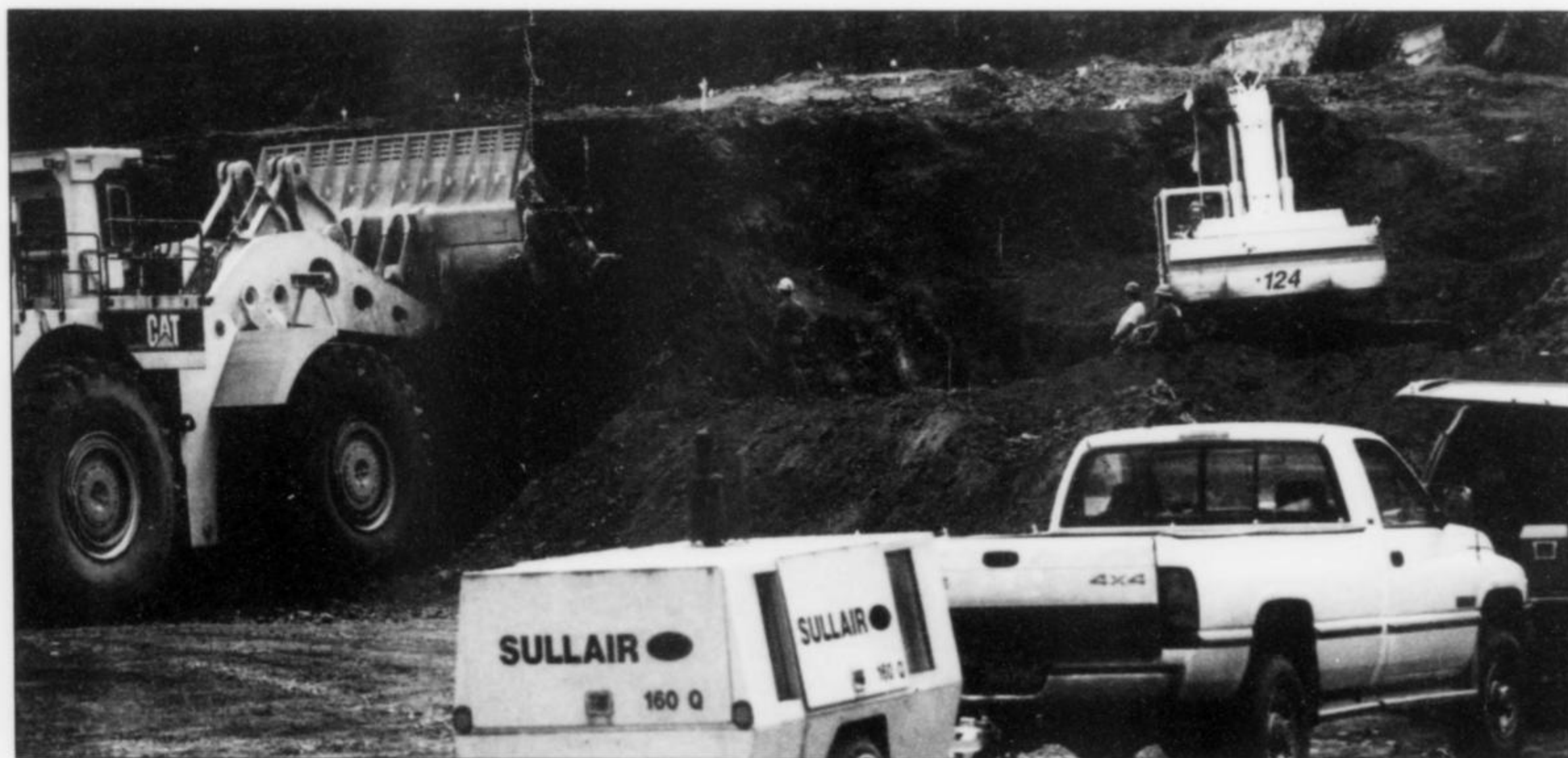
Figure 7. Collecting orpiment in the floor of the Mega pit; the orpiment zone here is about 25 feet wide and dips near-vertically.
