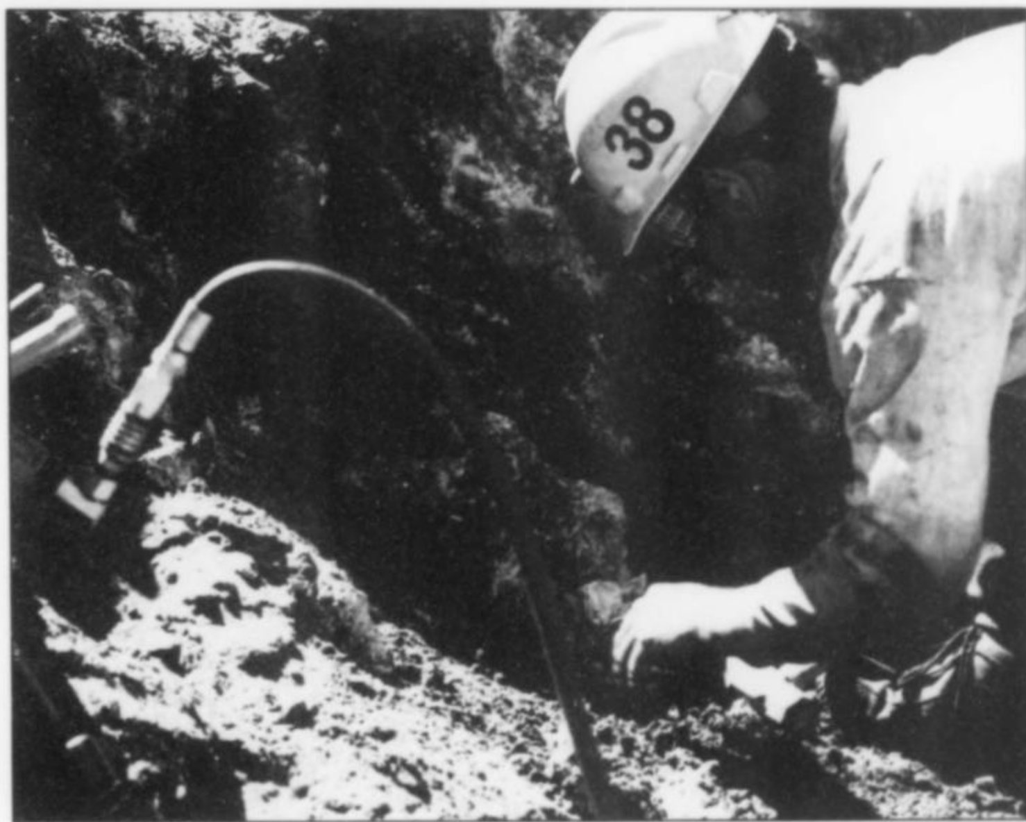
Figure 9. Graham Sutton working on an orpiment pocket in the Mega pit. Although the orpiment zone is 25 feet wide, individual pockets are generally less than 6 inches wide and 12 inches long. Great care is required to avoid bruising the soft crystals.
