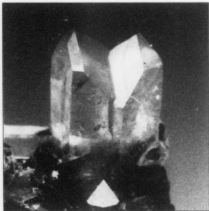
Figure 23. Quartz crystal, contact Dauphiné twin. RPR specimen #3186 and photo. Twinned crystal is 5 mm tall.
