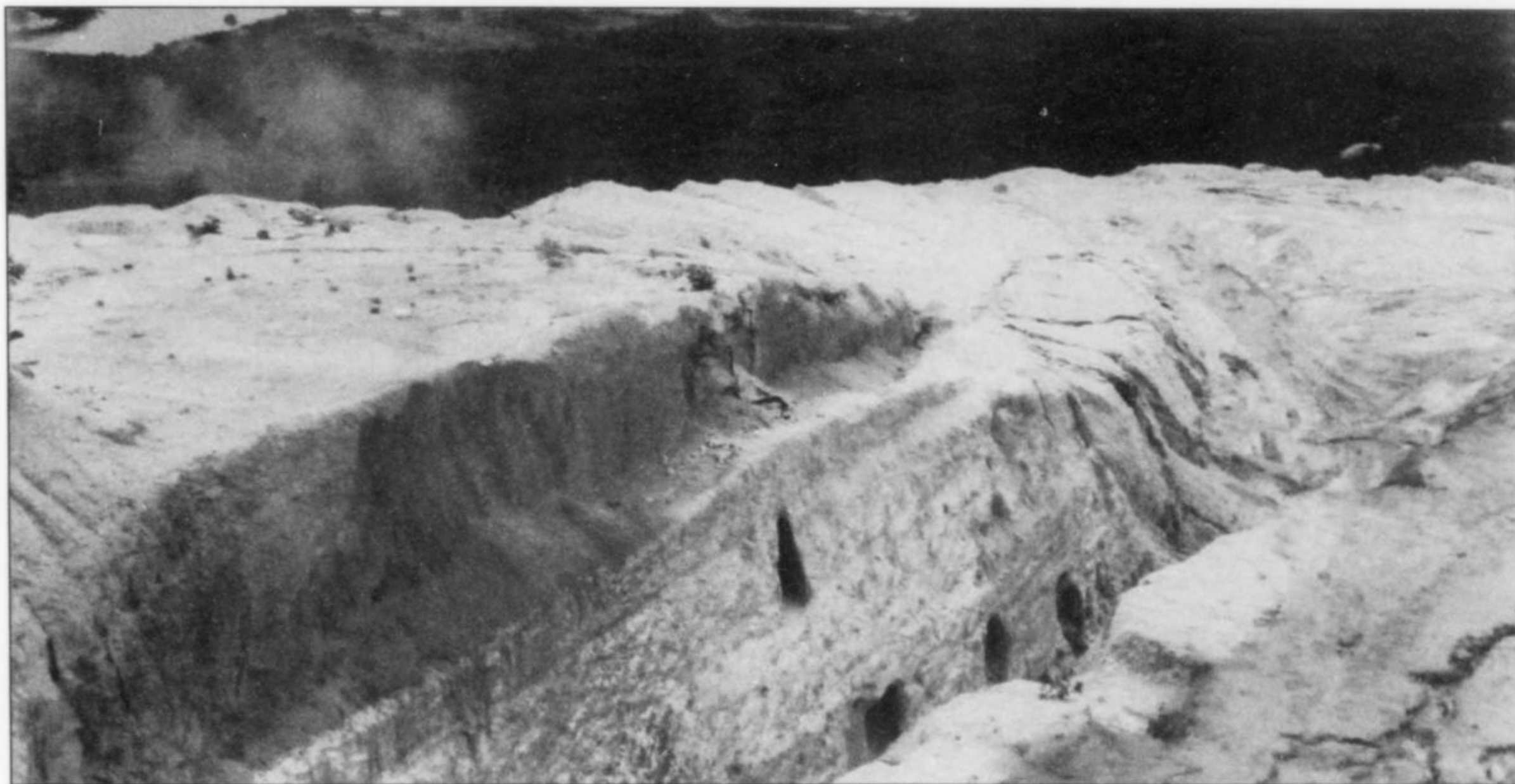
Figure 3. A deep open cut at the Cata Rica pegmatite shows holes dug in the walls where gem pockets containing tourmaline were found.
